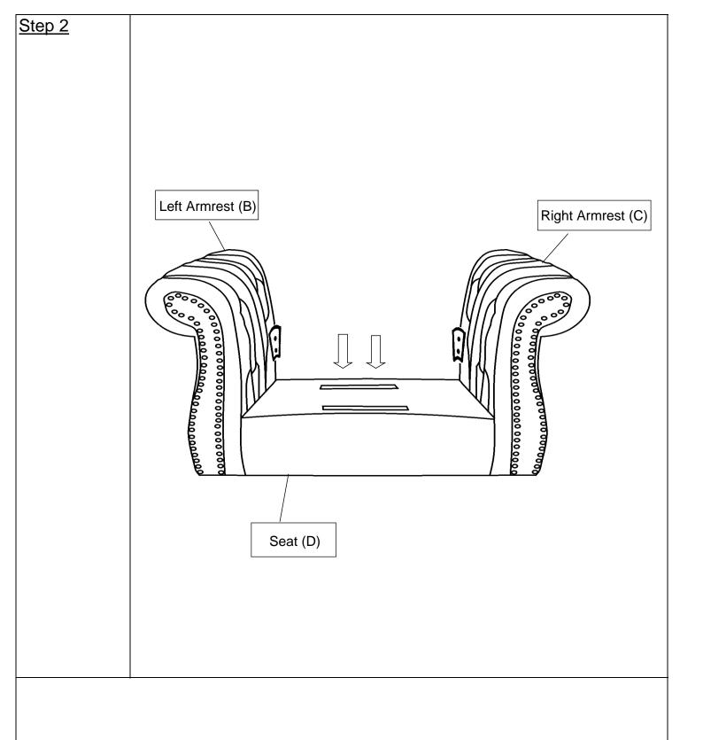
Push the Seat(D) downwards until it is fully slotted and locked into position in the Armrests.
