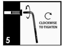
Make sure all parts are properly aligned, then use the appropriate hand tool to completely tighten the bolts or screws. Do not use power tools and do not overtighten.
