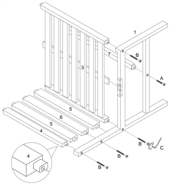
Insert part (5) into part (1) as per diagram, using bolt (A) insert into part (1) to part (7) ,and using bolt (B) into part (1) to parts (3,4,6) with hex key (C) as per diagram. Note: do not fully tighten all the bolts.
