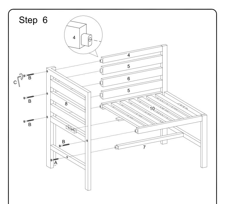
Repeat the last action as per diagram. Fully tighten all the bolts .
