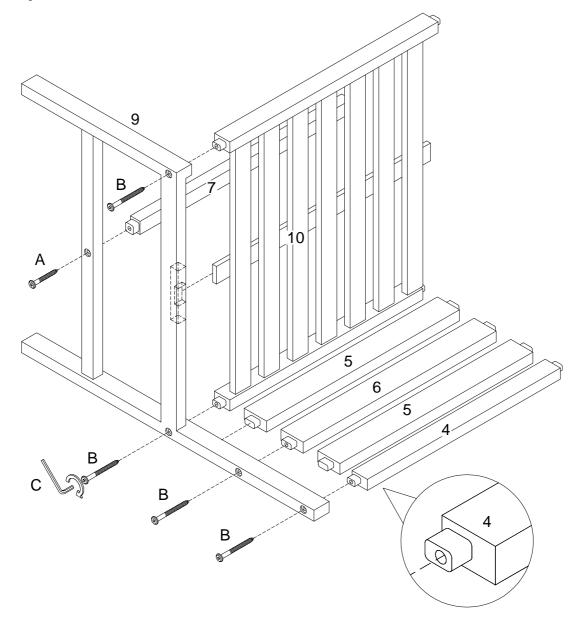
Insert part (5) into part (9) as per diagram, using bolt (A) insert into part (9) to part (7) ,and using bolt (B) into part (9) to parts (4,6,10) with hex key (C) as per diagram.
