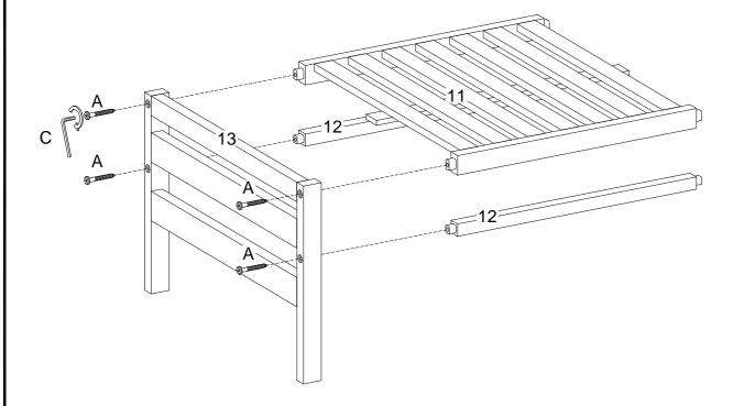
Using bolt (A) insert into part (13) to parts (11,12) with hex key (C) as per diagram. Note: do not fully tighten all the bolts .
