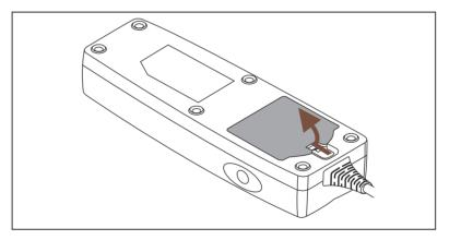
3. Insert two 9V batteries into the Power Converter. Do not use rechargeable batteries.
