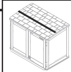
Align truss leg (L) to lid and lower into position. Attach truss leg (L) through pre-drilled holes, using ten screws (CC). Use force when starting to drive self-tapping screws. Once the screw pierces the plastic it will drive easier.
