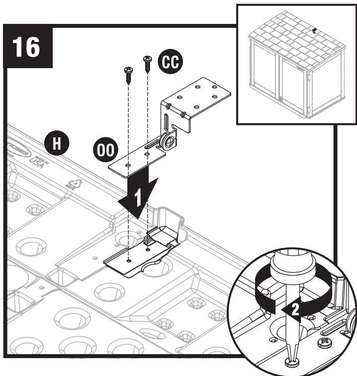
Install center hinge (OO) to lid (H) using two screws (CC).
