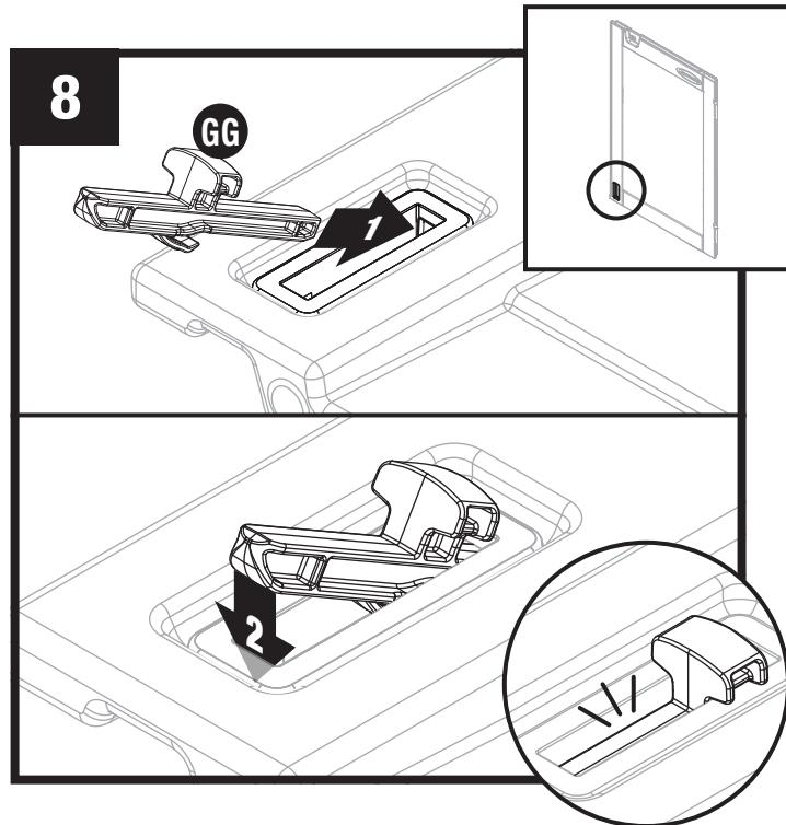
Insert door latch (GG) into door latch housing. Slide latch up and down to check if assembled correctly.
