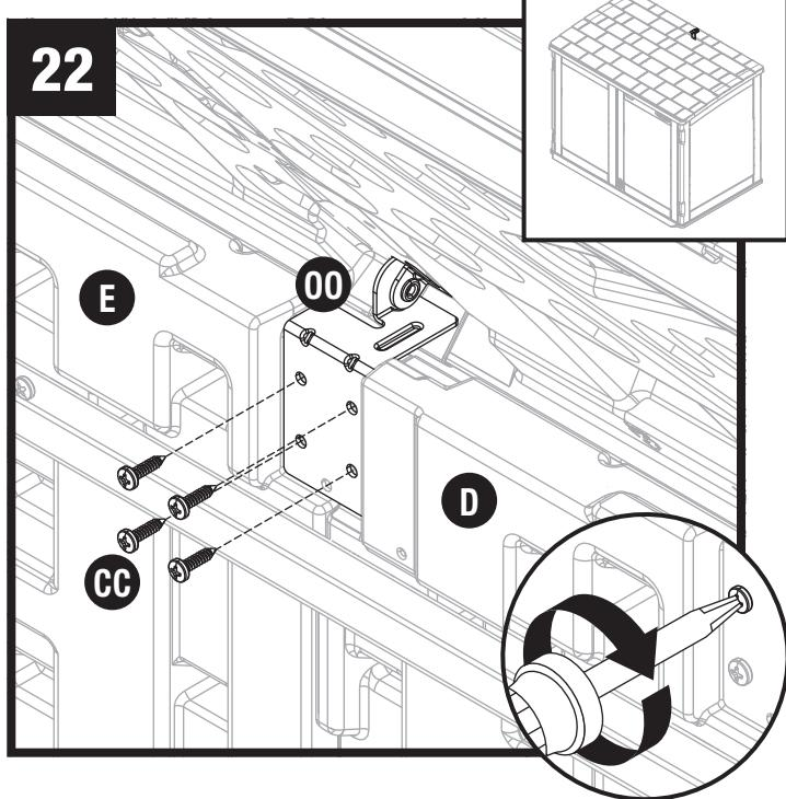
Secure center hinge (OO) to left and right back panels (E, D) using four screws (CC).
