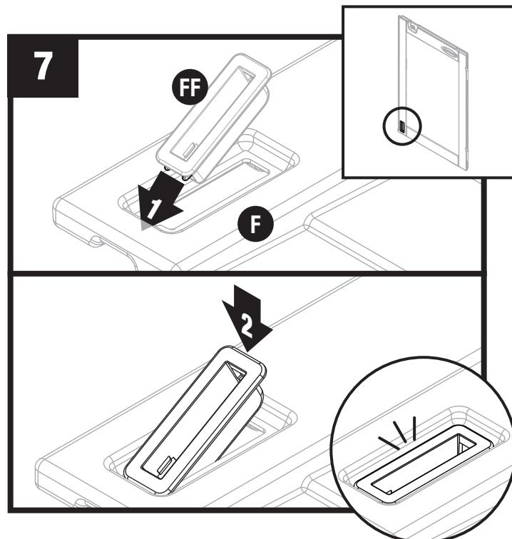
Insert door latch housing (FF) into right door (F) and snap into place.
