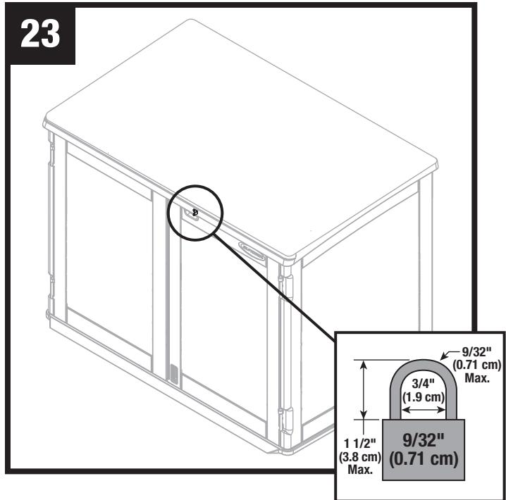
With roof closed, attach a 9/32" lock (not provided) to lock hasp (NN) to properly secure shed.
