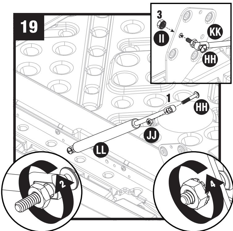
Insert bolt (HH) into shock (LL) bottom. Thread nut (JJ) onto bolt and tighten. Insert bolt (HH) into lower hinge (KK). On outer side of lower hinge (KK), install a second nut (II) onto bolt.
