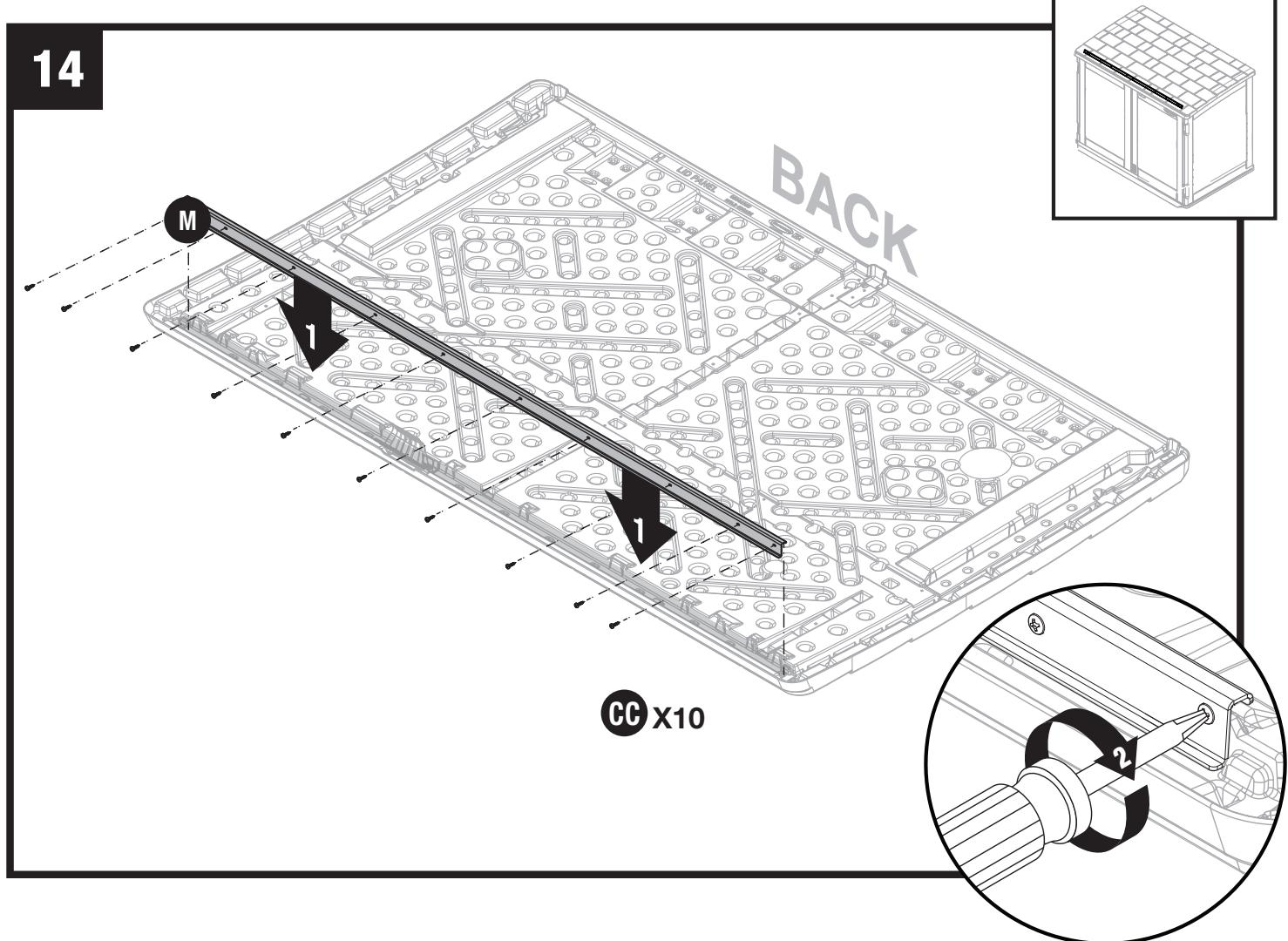
Lower front bracket (M) to lid. Attach front lid bracket (M) using ten screws (CC). Use force when starting to drive self-tapping screws. Once the screw pierces the plastic it will drive easier.
