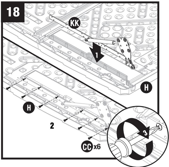
Lower hinge (KK) to lid panel (H). Nut should nest into pocket on lid. Attach hinge to lid panel by using six screws (CC). There are no pre-drilled holes on the lid. Use force when starting to drive self-tapping screws. Once the screw pierces the plastic it will drive easier.
