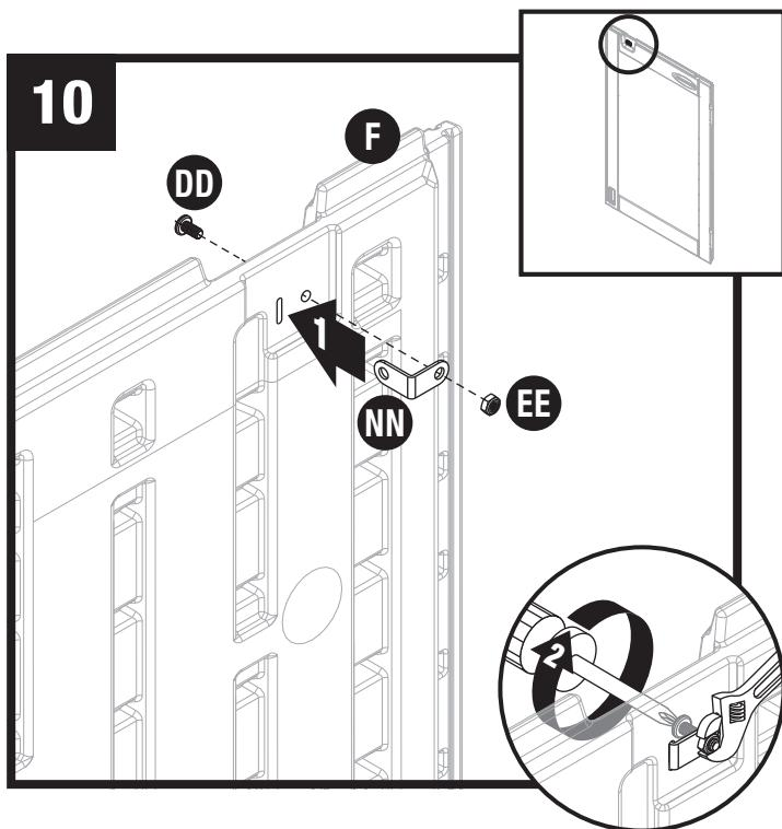
Attach lock hasp (NN) to right door (F) with one screw (DD) and one nut (EE).
