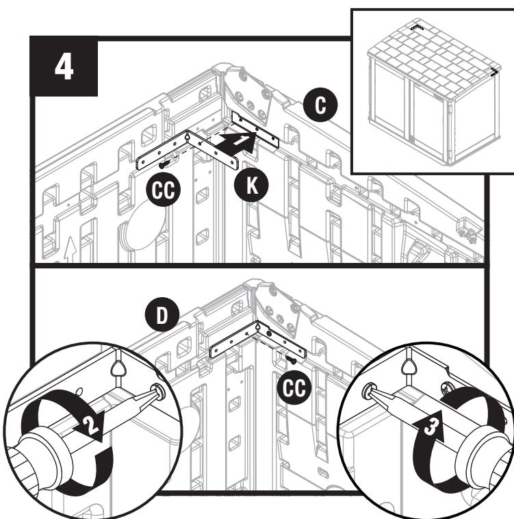
Attach a corner brace (K) to right panel (C) inner hole with screw (CC). Attach rear of corner brace (K) to right back (D) inner hole with screw (CC). Repeat for remaining corner brace (K), left panel (B) and left back (E).
