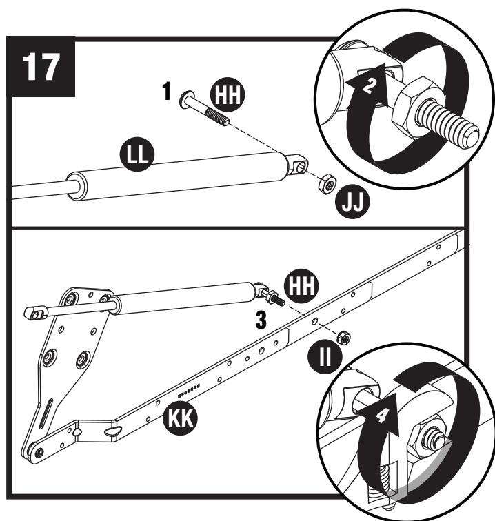
Insert bolt (HH) into hole in top of shock (LL). Thread nut (JJ) onto bolt (HH) and tighten. Insert bolt (HH) into hinge (KK). Use a wrench to tighten nut (II) onto bolt.
