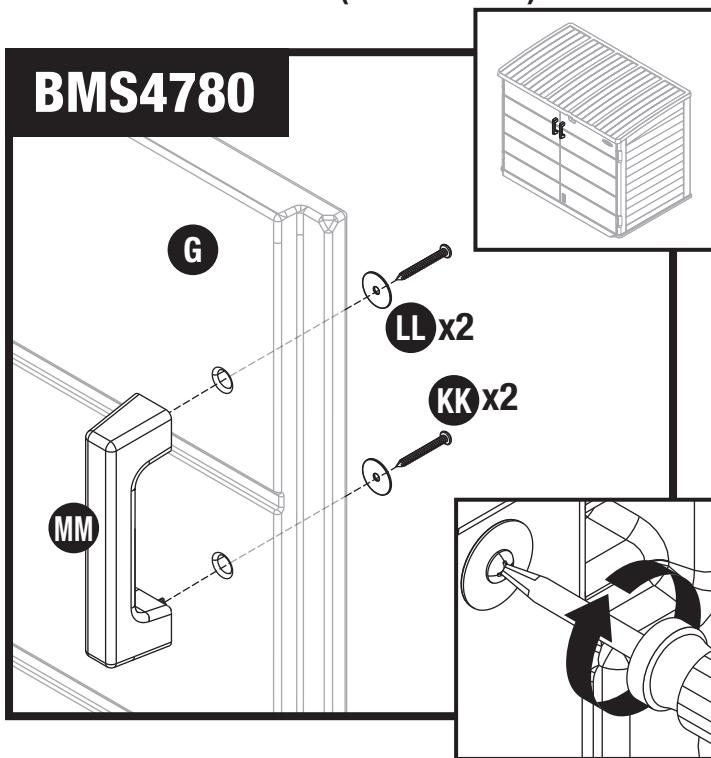
Install a door handle (MM) to left door panel (G) and secure using two washers (LL) and two screws (KK). Repeat for the right door panel (F).
