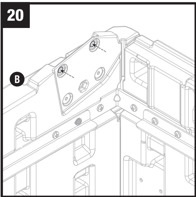
Cut or punch the top through holes on the left panel (B). Repeat for the right panel (C).
