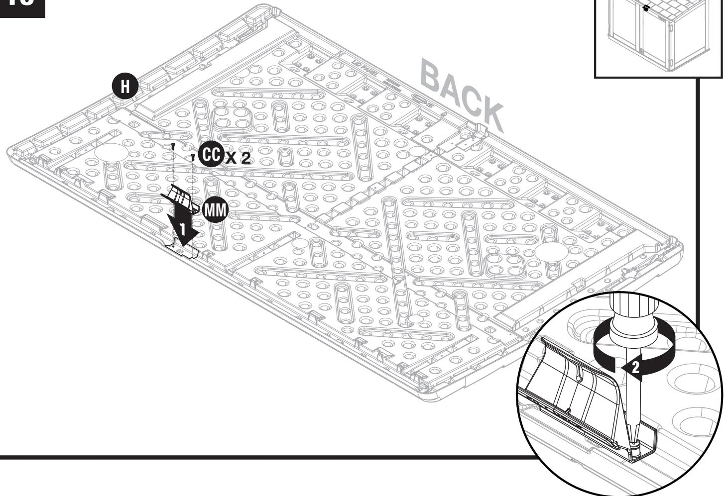
Lower lid latch (MM) to lid (H). Attach using two screws (CC).
