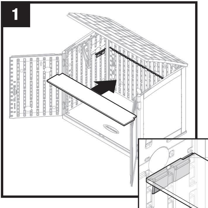
Place shelf into shed. Shelf must be completely seated into shelf supports on side and back panels.
