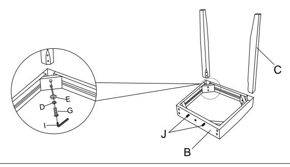
Attach the Chair back(A) to Seat(B) with Wood plug(J), then lock them using Lock washer(D), Flat washer(E), Bolt(F) and Bolt(H) by Allen key(I).
