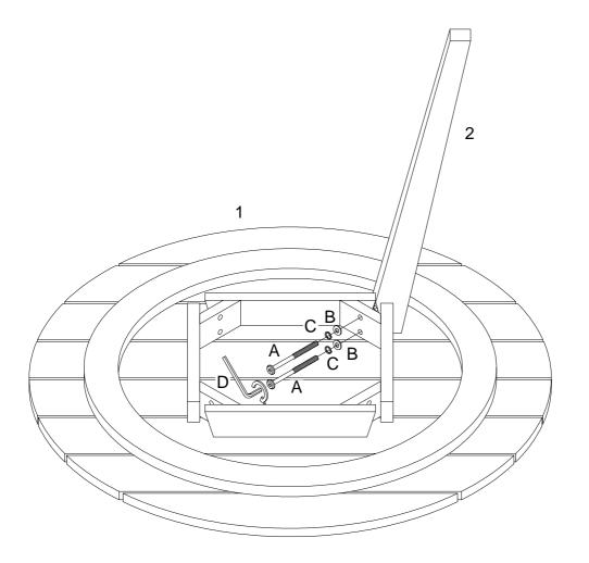
Fasten part (2) to part (1) by using bolt (A) with lock washer(C) and flat washer(B) with hex key (D)
