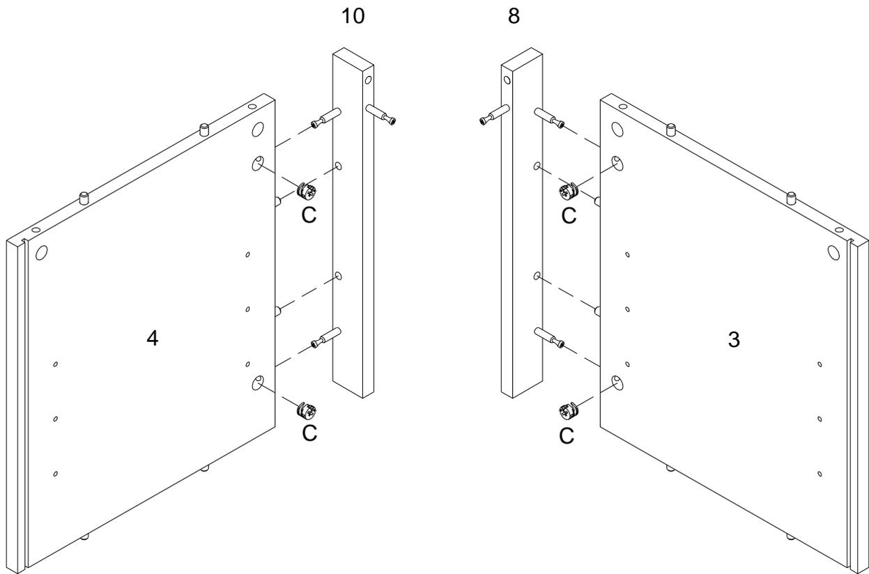
Using cam lock(C) secure part (10) into parts (4) ,part (8) into part (3) with Philips head screwdriver as per diagram.
