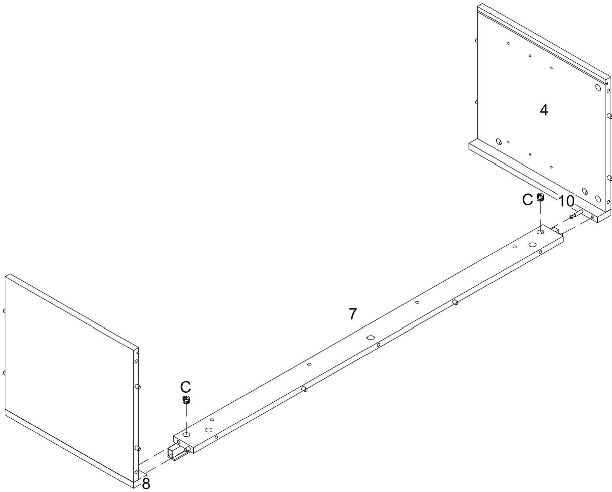
Using cam lock(C) attach parts (8,10) into part (7) with Philips head screwdriver as per diagram.
