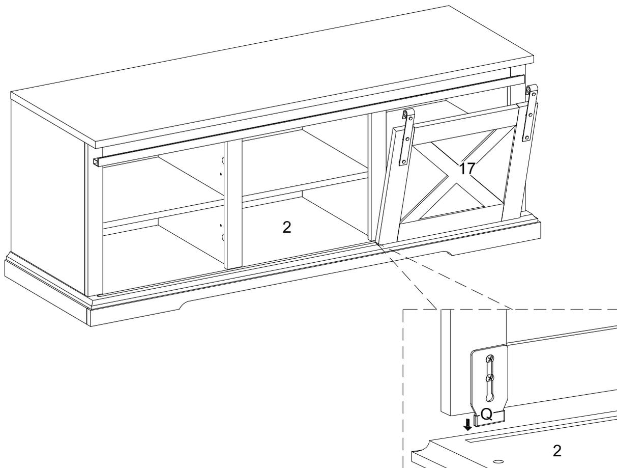
Place plate (Q) on door into groove.
