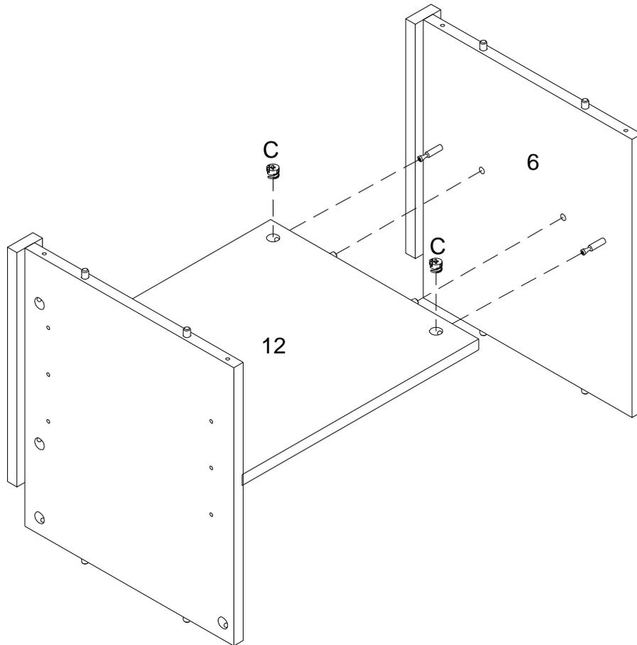
Using cam lock(C) secure part (6) into parts (12) with Philips head screwdriver as per diagram.
