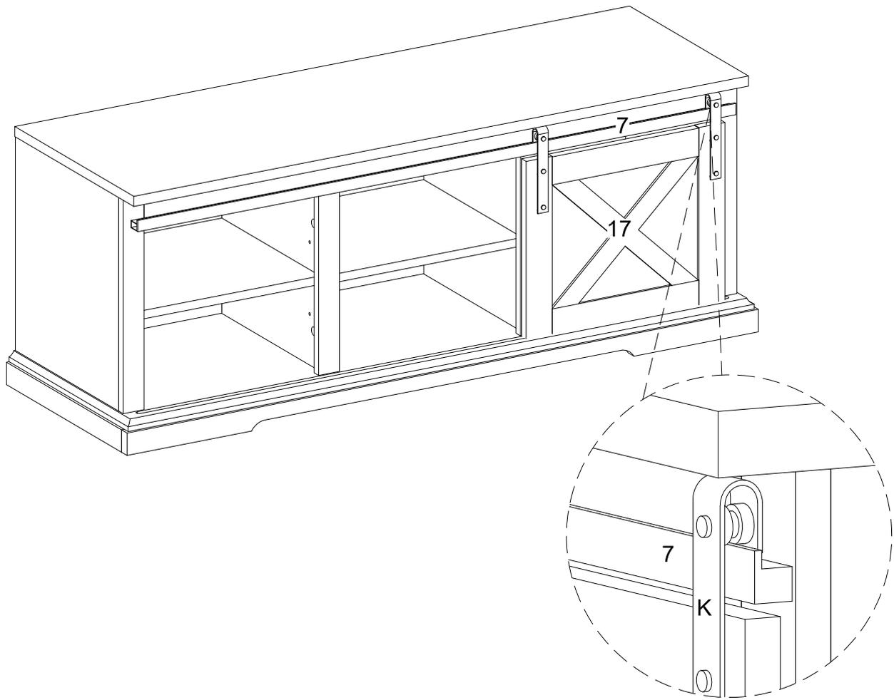
Hang pulley (K) to part (7), then press down to hold the door.
