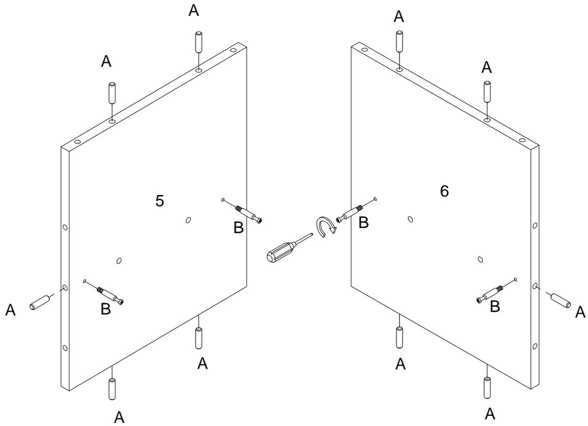
Insert wooden dowel (A) into parts (5,6), then secure cam bolt (B) into parts (5,6) with Philips head screwdriver as per diagram.
