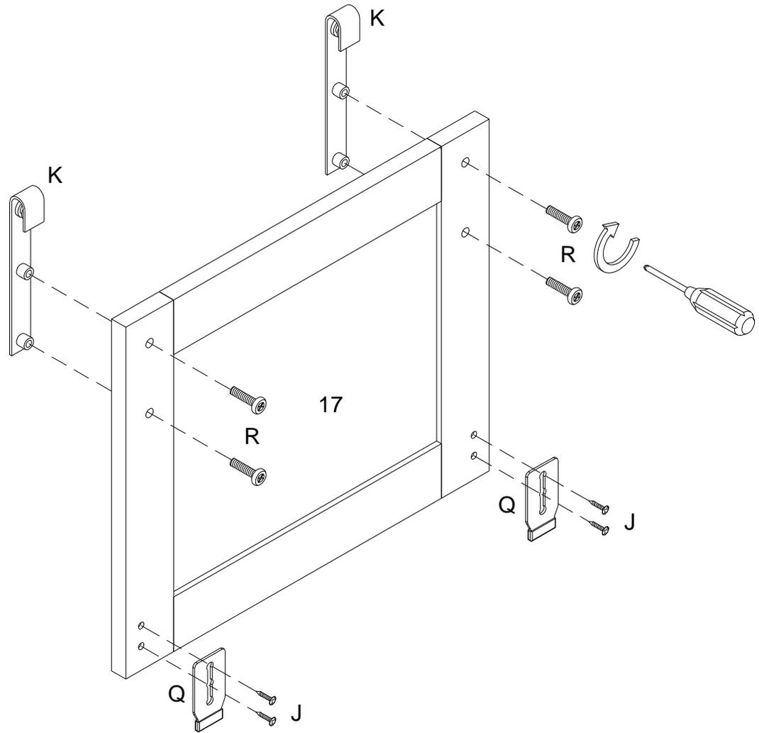
Using bolt (R) secure pulley (K) into part (17) ,then using screw (J) attach plate (Q) into part (17) with Philips head screwdriver as per diagram.
