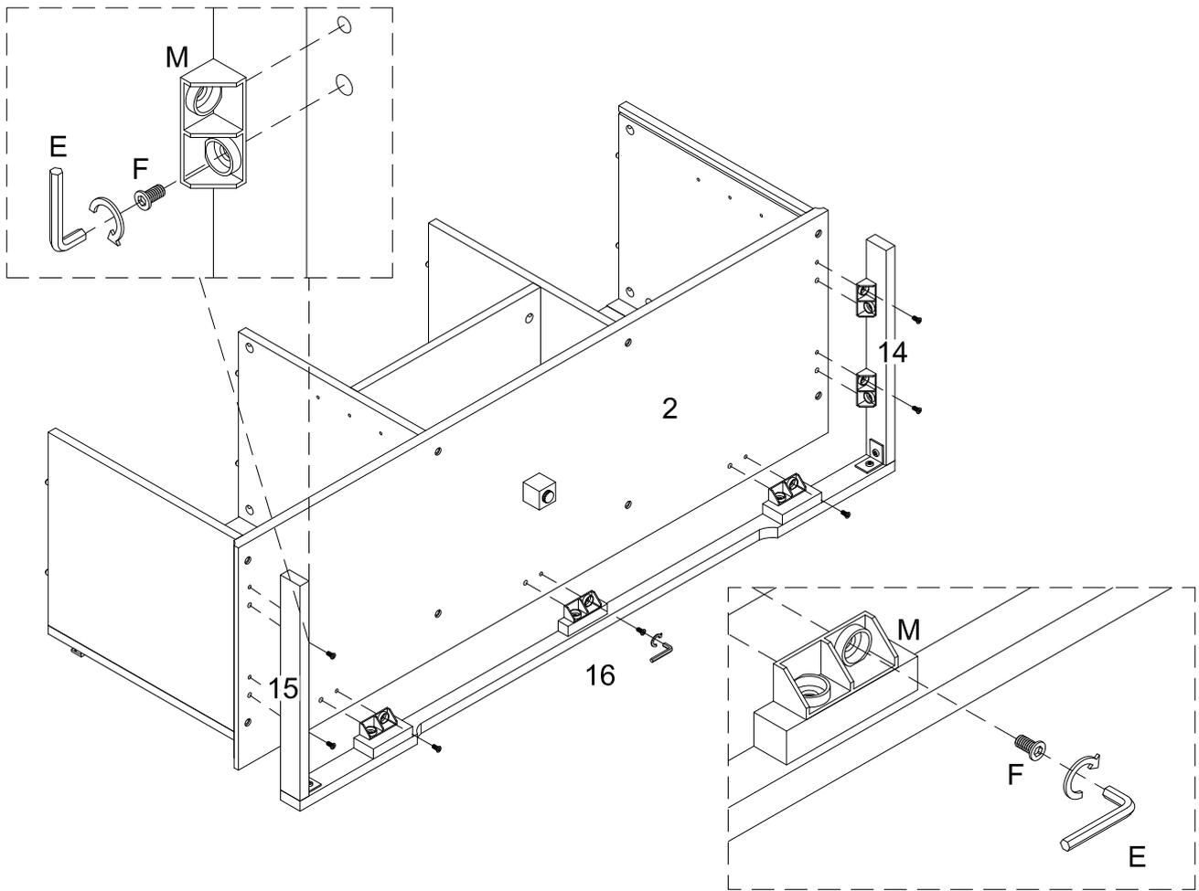
Using bolt (F) attach connector (M) to part (2) with hex key (E) as per diagram.
