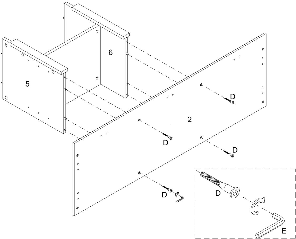
Using screw (D) attach part (2) into parts (5,6) with hex key (E) as per diagram.
