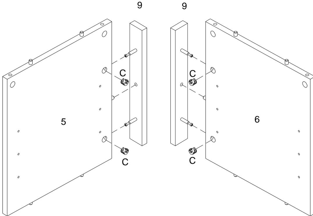
Using cam lock(C) secure part (9) into parts (5,6) with Philips head screwdriver as per diagram.
