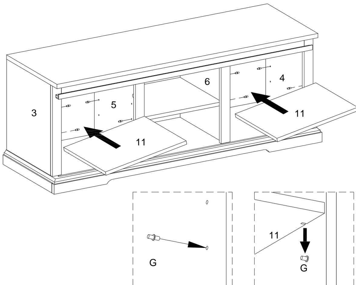
Insert shelf support pin (G) into parts (3,4,5,6) as per diagram. Make sure you place the four shelf support pins (G) in the same level. So the shelf is not titled .Put part (11) into unit as per diagram. Tilt and rest the adjustable shelf(11) onto the shelf support pins .
