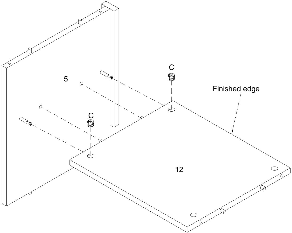
Using cam lock(C) secure part (5) into parts (12) with Philips head screwdriver as per diagram.
