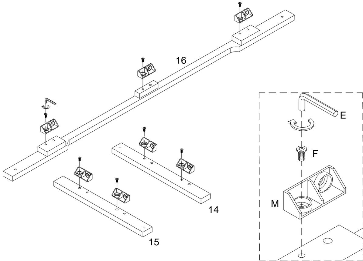
Using bolt (F) attach connector (M) to parts (14,15,16) with hex key (E) as per diagram.
