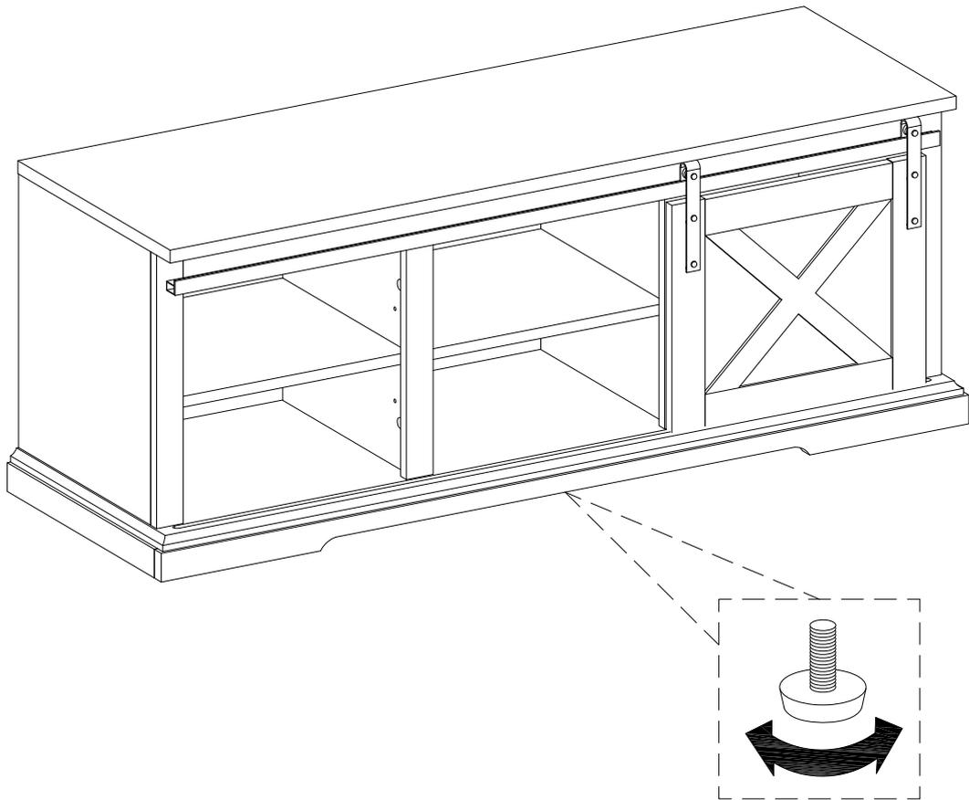
if necessary, adjust the pre-attached Floor Levelers at the bottom to level the unit.
