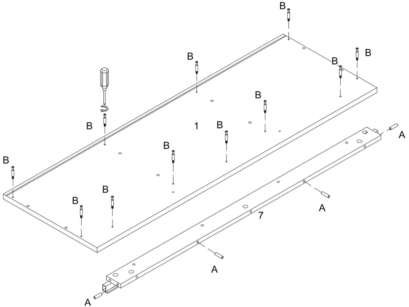
Insert wooden dowel (A) into part (7), then secure cam bolt (B) into part (1) with Philips head screwdriver as per diagram.
