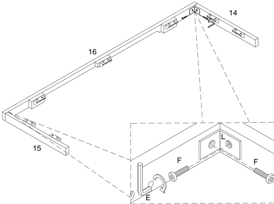
Using bolt (F) attach connector (L) to parts (14,15,16) with hex key (E) as per diagram.
