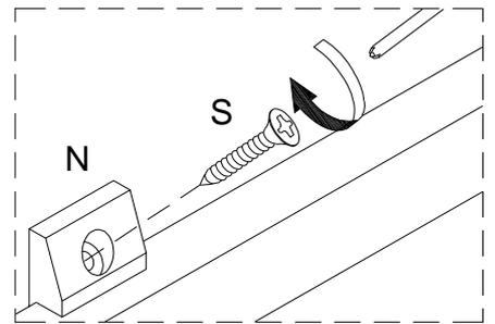
Using screw (S) secure plastic wedge (N) to part (13) with Philips head screwdriver as per diagram.
