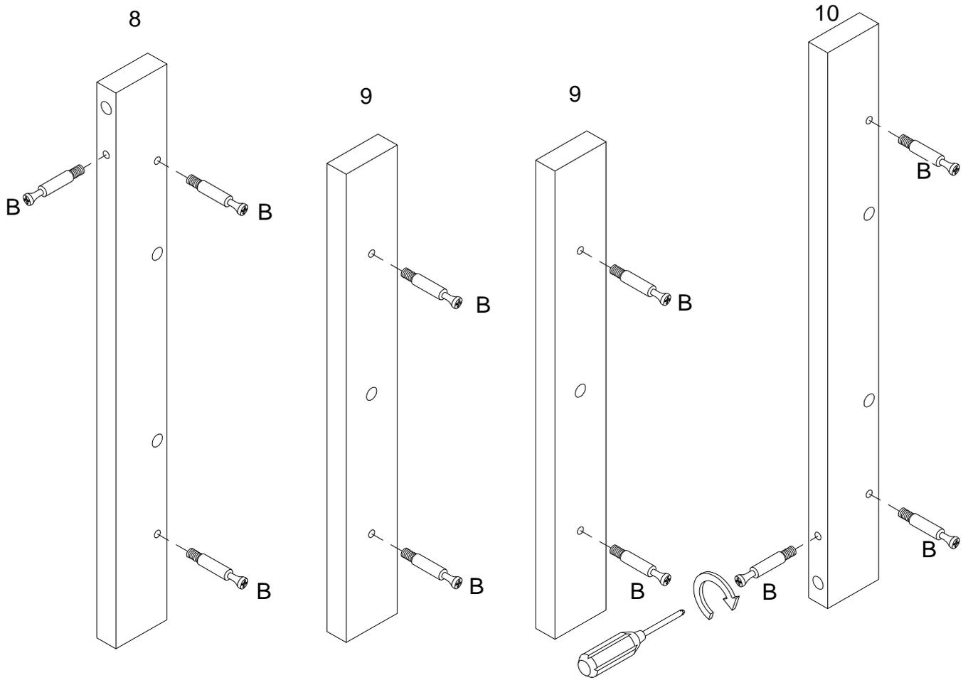
Secure cam bolt (B) into parts (8,9,10) with Philips head screwdriver as per diagram.
