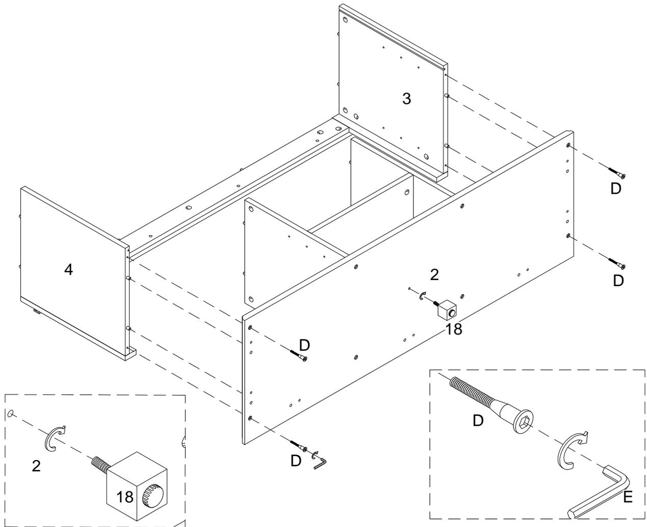
Secure part (18) into part (2), then using screw (D) attach part (2) into parts (3,4) with hex key (E) as per diagram.
