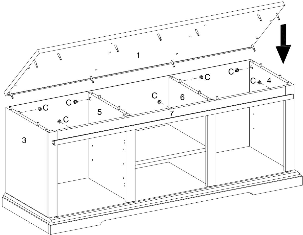
Using cam lock(C) secure part (1) to parts (3,4,5,6,7) with Philips head screwdriver as per diagram.
