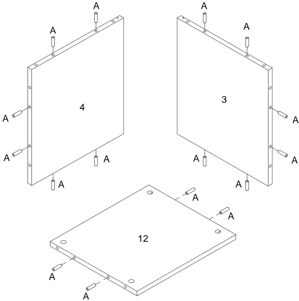
Insert wooden dowel (A) into parts (3,4,12) as per diagram.
