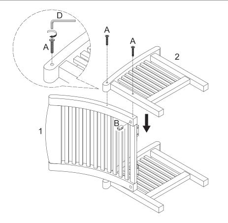
Insert barrel nut (B) into chair back (1). Attach chair side (2) to chair back (1) using bolts (A). Tighten bolts (A) with wrench (D).
