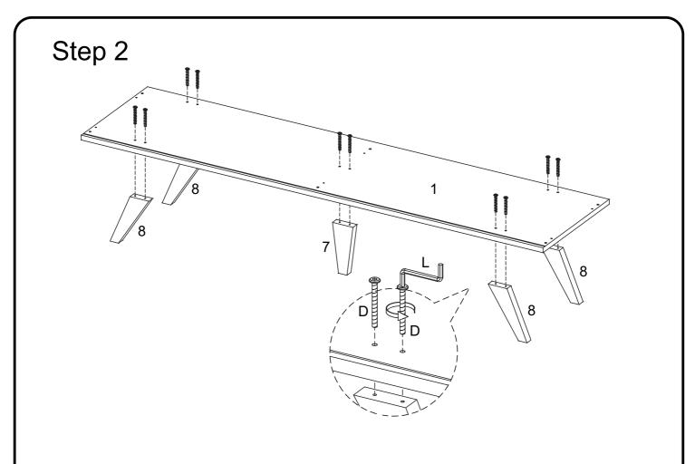
Attach feet (7,8) to base panel (1) with screw (D) and hex key (L).
