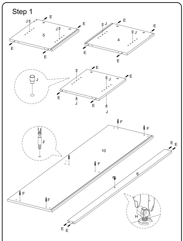
Insert wood dowels (E) into the indicated parts. Screw Cam Bolt (F) into top panel (10). Place shelf support pins (J) into right and left side panels (4,5) and into both sides of divider panel (3) as shown. Insert plastic support (H) into front rail (6).
