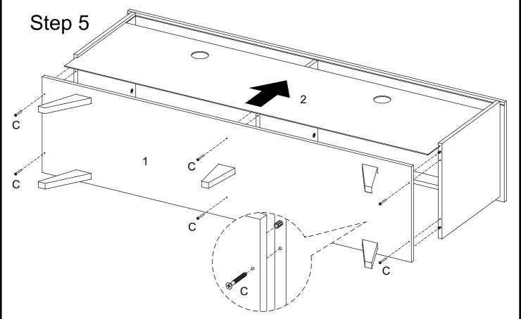
Insert back panel (2) into grooves on side panels (4) (5) and top panel (10). Secure base panel (1) to side panels (4) (5) and center panel (3) with screw (C) and screwdriver (not included).
