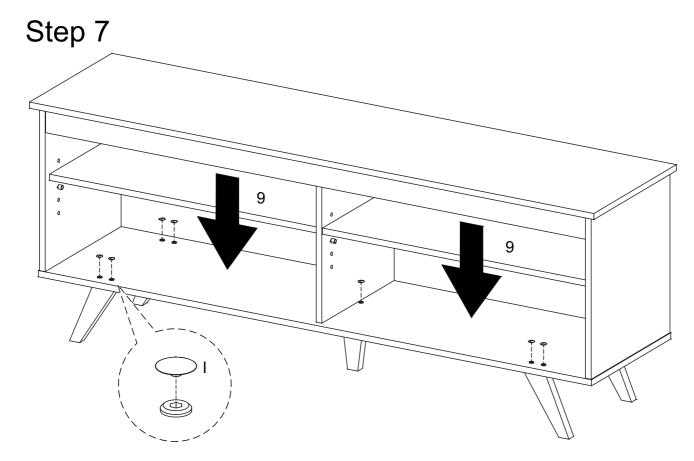
Use plastic cap (I) to cover screw heads (D) as desired. Place the shelves (9) onto the support pins already fixed, as shown.
