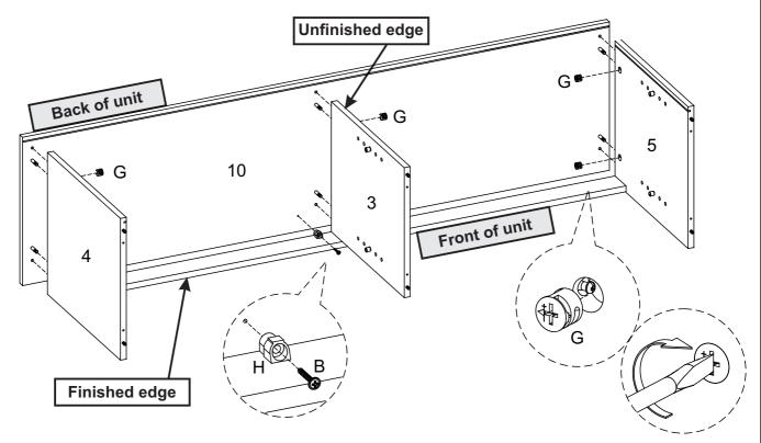
Fit side panels (4) (5) and middle panel (3) to top panel (10) as shown. Secure cam locks (G) where shown, with screwdriver (not included). Use screw (B) to secure to top panel (10) through plastic support (H).
