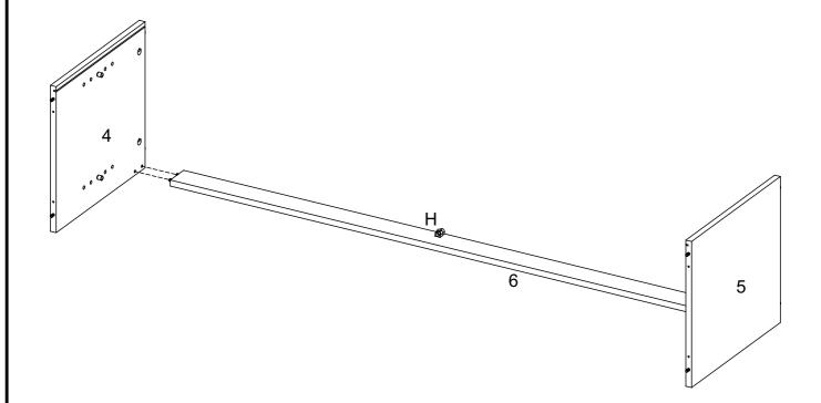
Join front rail (6) between the side panels (4) and (5) as shown. Note the position of part (H) for correct fit.
