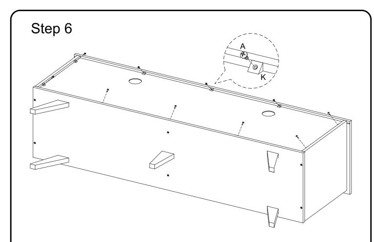
Secure back panel (2) with screw (A) and back support (K) with screwdriver (not included).
