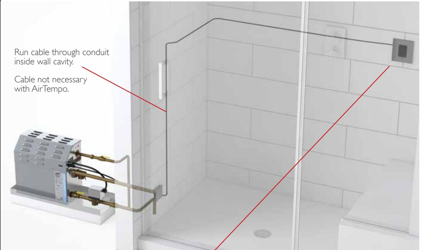
Run cable through conduit inside wall cavity.
