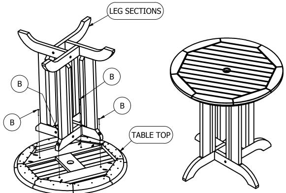
**5)** Step 5: Attach Leg Sections to Table Top with (4) "B" Bolts.
