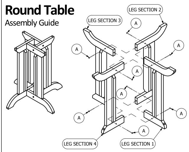
**NOTE:** All 4 Leg Sections are Identical and Numbered for Order of Assembly Only.
