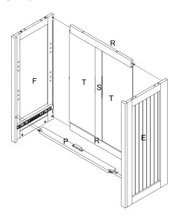
Step 7. Attached bottom panel (part B) to lower left side panel (part E), lower right side panel (part F) and back rail (part R) using wood dowels (part #7), long hex socket head bolts (part #1), spring washers (part #9), flat washers (part #10) and allen wrench (part #15). NOTE: Please fully tighten bolts at this time.
