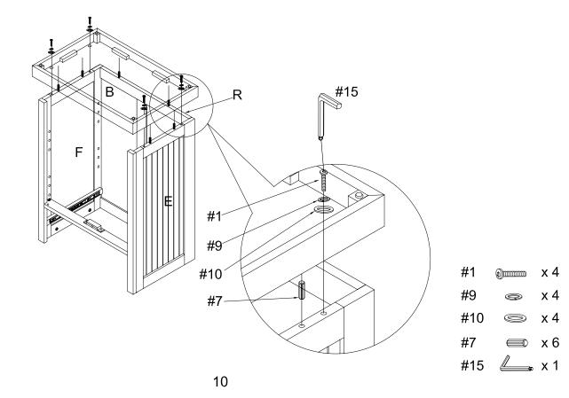
Step 8. Carefully lay the assembled top and bottom cabinets as shown, and attach them together using short hex socket head bolts (part #2), spring washers (part #9), flat washers (part #10) and allen wrench (part #15).
