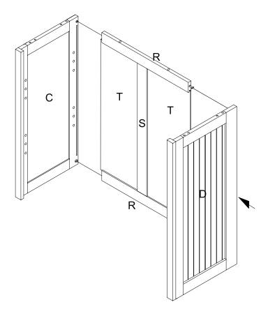
Step 4. Attach top panel (part A) to upper left side panel (part C), upper right side panel (part D) and back rail (part R) using wood dowels (part #7), long hex socket head bolts (part #1), spring washers (part #9), flat washers (part #10) and allen wrench (part #15).
