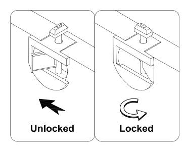
Reference the images above any time the instructions state "lock the hardware". Note: Be sure to check all hardware is locked when completed.
