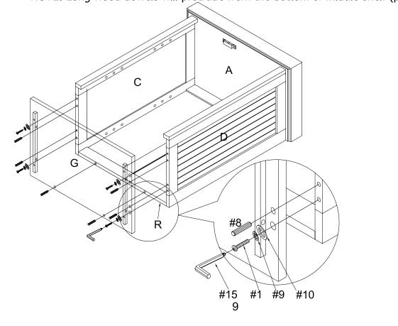
Step 6. Attach lower left side panel (part E) and lower right side panel (part F) to back rails (part R) and front rail (part P) as shown and lock the hardware.
