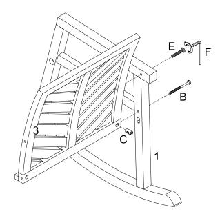
Attach part (3) to part (1) using bolt (B, E) and nut (C) with hex key (F).
