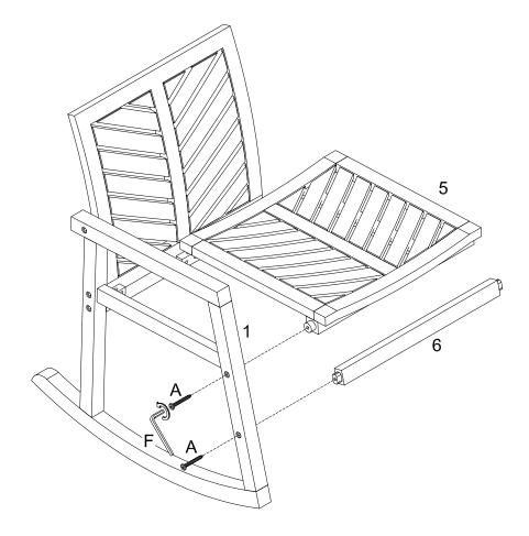
Attach part (5, 6) to part (1) using bolt (A) with hex key (F).
