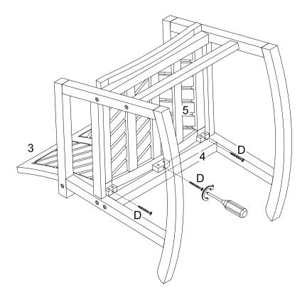
Lay down chair, secure part (3, 4, 5) using screw (C) as per diagram.
