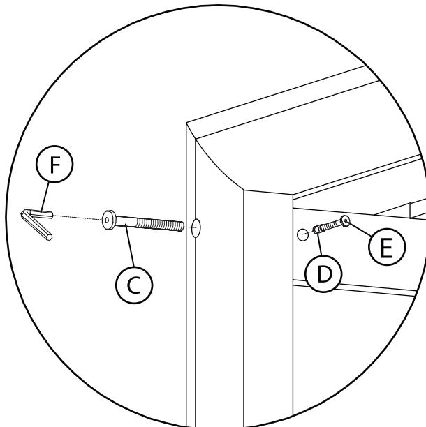
**NOTE:** Use bolt (E) as an extension to insert barrel nut (D) into the hole found on the ottoman base (A). Screw the bolt into the top of the barrel nut. Once bolt (C) is secured through the frame and into the barrel nut (D), remove bolt (G) from barrel nut (D).
