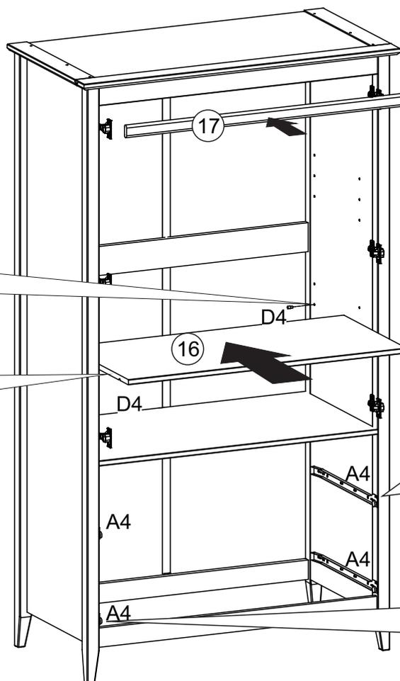
Attention: There are no predrilled holes for the A4 screws on parts 02 and 03.
