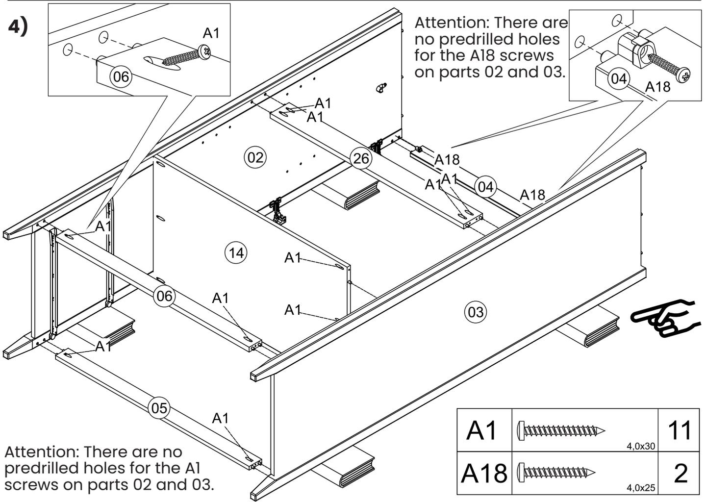
Attention: There are no predrilled holes for the A18 screws on parts 02 and 03.
