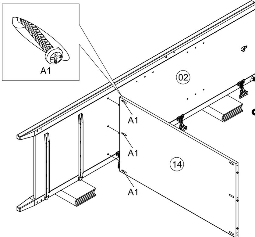
Attention: There are no predrilled holes for the A1 screws on part 02.
