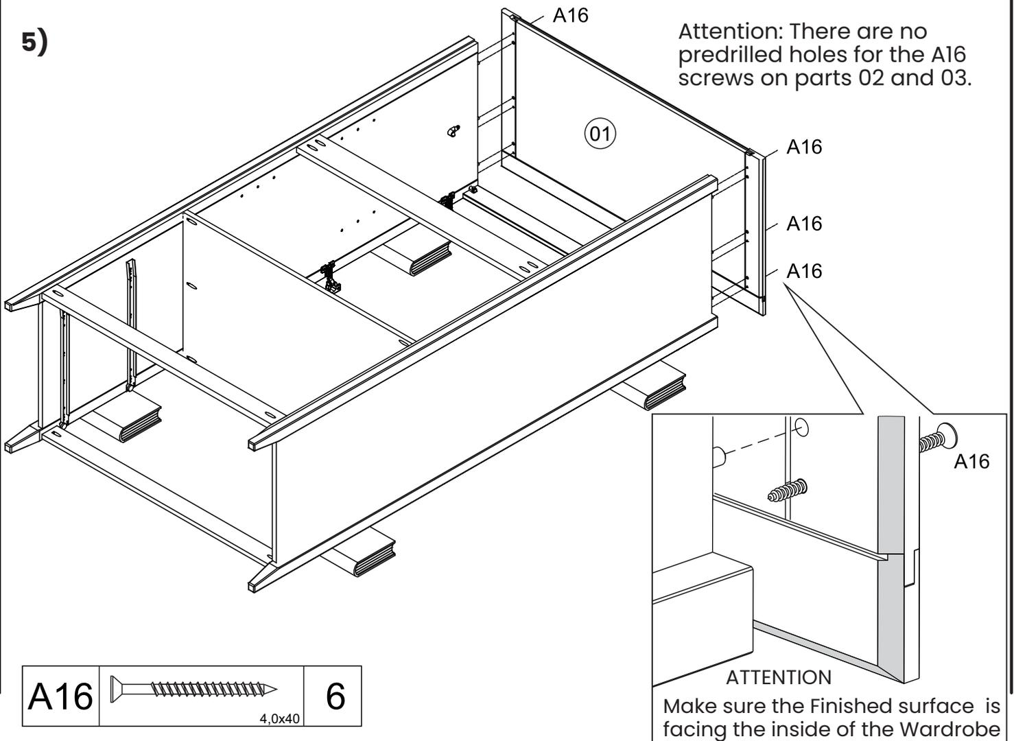
Attention: There are no predrilled holes for the A16 screws on parts 02 and 03.
