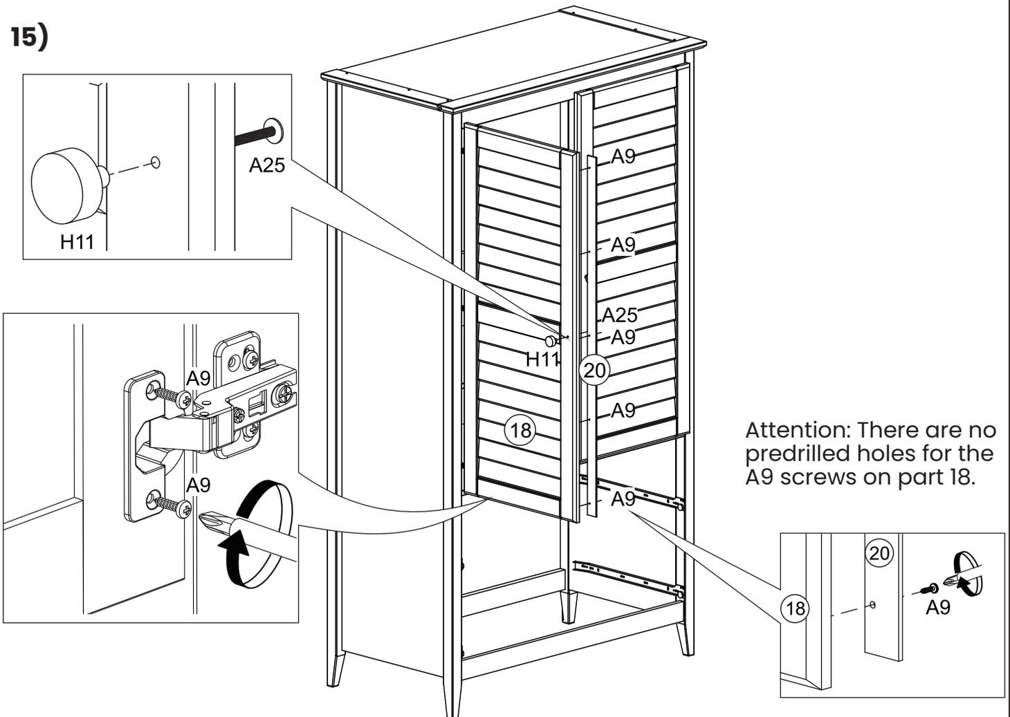
Attention: There are no predrilled holes for the A9 screws on part 18.
