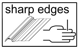
Care must be taken when handling various pieces of your building since many contain sharp edges. Please wear work gloves, eye protection and long sleeves when assembling or performing any maintenance on your building.
