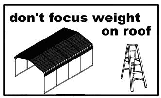
NEVER concentrate your weight on the roof of the building. When using a step ladder make sure that it is fully open and on even ground before climbing on it.
