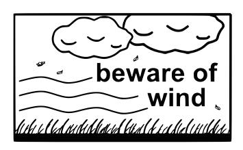
Do NOT attempt to assemble your building on a windy day. The large panels can catch the wind like a "sail", causing them to be whipped around making construction difficult and unsafe.
