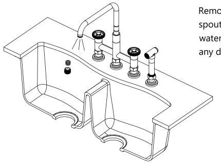
Remove the aerator from the spout. Turn faucet on and let the water run for 60 seconds to flush any debris.
