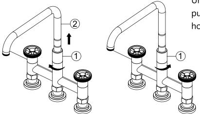
Unthread the holding nut (1) and pull the spout (2) up. Thread the holding nut (1).
