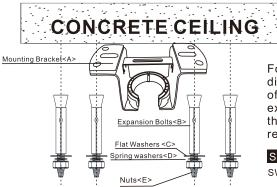
Note: According to the ceiling of different materials, use different screws to fix the hanging bracket.  $\triangle$ To both the hanging bracket on the wood ceiling less than 12MM to prevent danger caused b loosening of screws. After the hanging bracket is completed, ensure that it can withstand the tension test of more than 68KG for safety.
