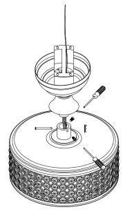
The first step of the suspension motor. E12 MAX40W\*3PCS 1. Unscrew the three screws of the motor cover. 2.Screw the E12 bulb with the appropriate wattage into the socket. 3. Insert the motor outer cover into the motor and tighten the screw. temos
