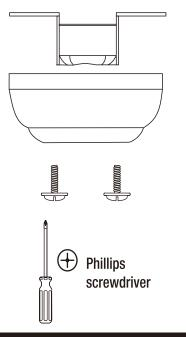
1:Remove the mounting bracket from the canopy by loosening the two canopy screws located in the L shaped slots. 2:Remove and save the two canopy screws in the round holes. This will enable you to remove the mountingbracket
