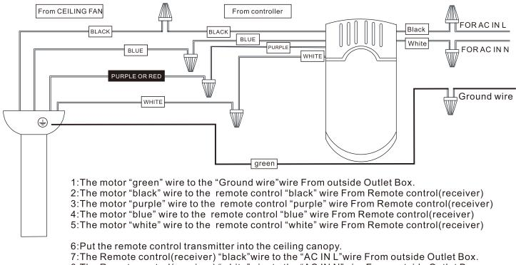
7:The Remote control(receiver) "black"wire to the "AC IN L"wire From outside Outlet Box. 8:The Remote control(receiver) "white"wire to the "AC IN N"wire From outside Outlet Box. 9:Use the remote control to start using the ceiling fan lamp.
