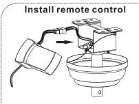
Carefully push the canopy to the bottom of the mounting bracket, make two sliding holes aligned to the two promine screws on the mounting bracket, and then turn clockwise until tight.
