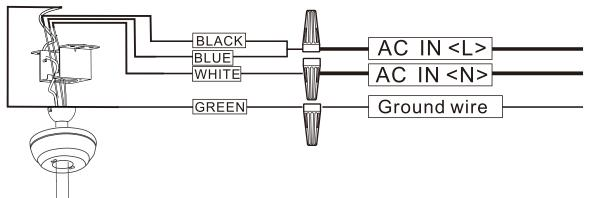
1. The motor "green" wire to the "Ground wire" wire from outside Outlet Box.
