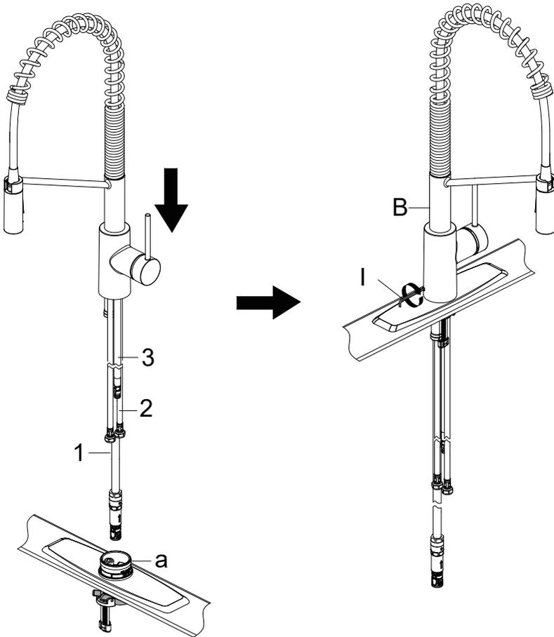
Insert the hose (1), supply lines (2) and quick connect hose (3) one by one through the hole of the base (a). Carefully insert the hoses into the base. Place the faucet assembly onto the base (a) as shown in the above figure. Secure the faucet assembly (B) by tightening the set screw with the provided hex wrench (I, Hex: 2.5 mm).
