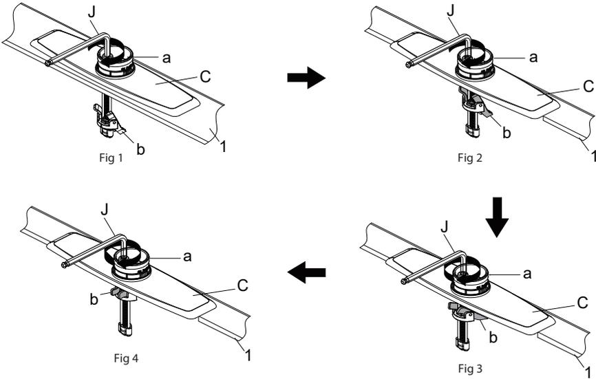
Press the base (a) and escutcheon (C) so that they can not move, then turn the screws with the provided hex wrench (J, HEX: 6.0mm) clockwise, as shown Fig 1. When the mounting plates (b) make contact with the sink (1), continue to turn the screw with the provided hex wrench (J, HEX: 6.0mm) clockwise, as shown Fig 2, until the base (a) is completely tightened and secured, as shown Fig.4.
