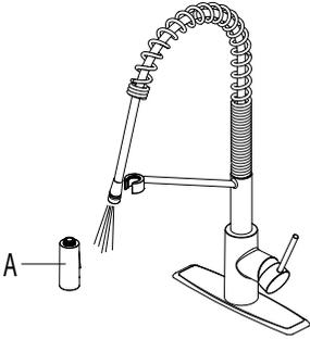
**NOTE:** Please make sure washer is installed attaching sprayer to hose.
