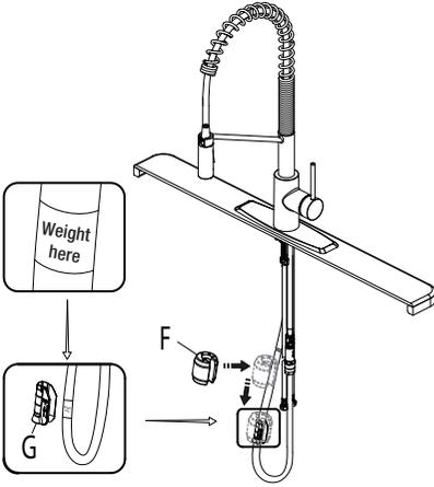
Install the weight clip (G) at the point of the hose marking "weight here". Insert the weight (F) onto the weight clip (G) by sliding it down onto the weight clip (G).
