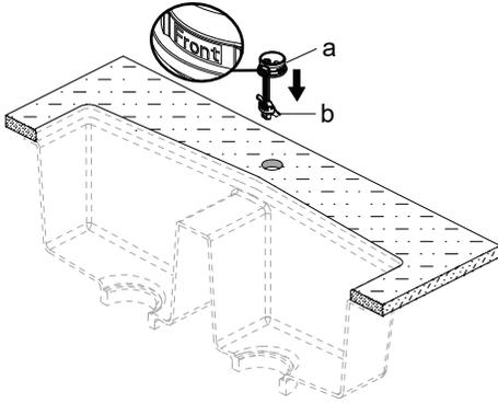
Shut off the water supply. Remove the old faucet. Clean the mounting surface. Check for the proper thickness of the sink. Insert the base (a) into sink. If your model does have a escutcheon, skip to step 1 b.
