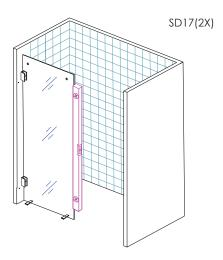
**Step 5** - Measure the width of the fixed panel and place the 1/8" thick rubber blocks provided 3" in from each end where the glass panel will sit on the tile / pan. Gently place down the glass panel on the rubber blocks & slide glass into the wall brackets. Check the glass is level, if not adjust by adding thinner 1/16" rubber block to the blocks already placed on the floor. Once level tighten the grub screws very tight on the wall brackets
