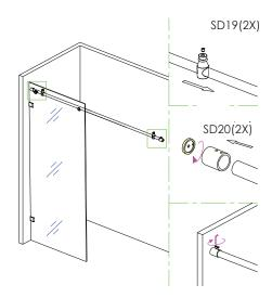
**Step 8** - Using 1/4" drill bit, drill holes and install wall plug. On one wall install only the round flat fixing piece with rest of bracket remaining on rod. On the second wall install the complete bracket. This allows you to slide the rod into one whole bracket and then screw remaining bracket on at opposing wall. Re-check the rod and glass and fixed panel are level then tighten the brackets on fix panel very tight.
