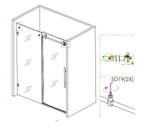
**Step 12** - Adjust Parts SD 19 door stops on top of shower rod to ensure the door panel does not hit the wall or the door handle touches the fixed panel.
