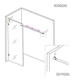
**Step 7** - Install the brackets on shower rod into the holes on the fixed panel. Using a level, check rod is perfectly level from one wall to the other. Once in correct position mark the placement of brackets on wall and uninstall rod from glass panel. Remove one of the wall brackets from rod and mark the holes to be drilled on each wall.
