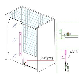
Step 9 - Make sure both ends of the fixed panel are the same distance to the front of the threshold tile and check panel is level again. Measure 1 1/8" from the front edge of glass towards the inside of shower - this is placement for the inside edge of the floor bracket as shown in diagram above. Mark holes on curb for floor bracket, drill 1/4" holes and instal floor bracket part SD18. Important - Check plastic piece in floor bracket is set to 10mm (3/8") glass.
