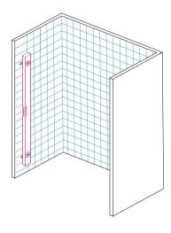
**Step 2** - Measure the width of threshold tile where shower door is to be installed, this needs to be a minimum of 2 3/4" to instal this model shower enclosure. On the wall where the fixed panel is to be placed measure to the centre of the threshold tile, from here measure back toward the front of shower 1 1/8" and mark the wall with a pencil. Using a level draw a line up the wall at this point.
