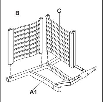
Attach back support (B), and seat (C) into right side frame (A1) to the matching holes.
