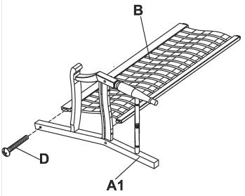
Attach back support (B) into right side frame (A1) to the matching holes, secure using 1 1/2" bolt (D).
