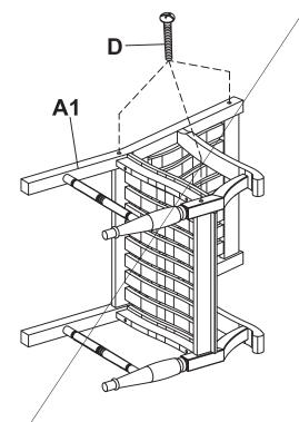
Turn the chair onto the other side and repeat step 2 to fasten the right side frame (A1).
