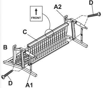
Attach the seat (C) and left side frame (A2) to the pre-assembled and secure using 1 1/2" bolts (D).
