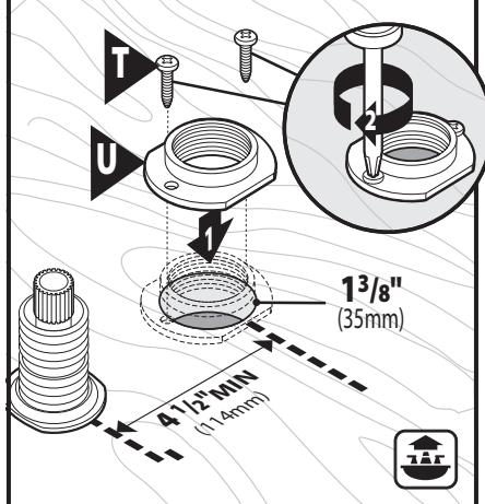
Attach Threaded Shank Adaptor (U) to the deck with 2 Screws (T).
