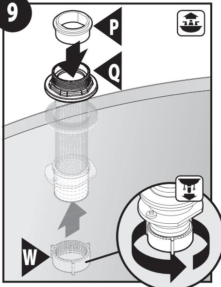
Insert Upper Hose Guide Washer (P) into Hose Shank Assembly (Q). Thread Lower Guide Washer (W) onto Brass Shank.
