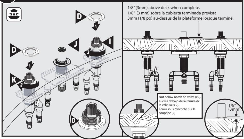
Thread Top Mounting Nuts (D) onto Spout Shank Body (J) and onto Hot and Cold Valve Bodies (I & K). Top nuts (D) are below the groove on each valve when properly assembled. On center shank leave 1/8" of threads above deck.
