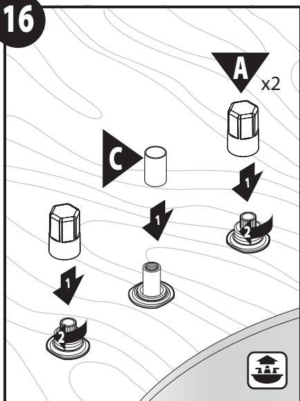
Place Protective Tubing (**C**) over center Shank Assembly (**J**) and Protective Caps (**A**) over Valves (**I & K**). Install test plug (**B**).
