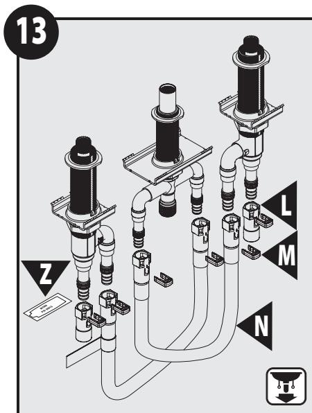
Apply Grease (**Z**) to all O-rings. Slide the Quick Connect Flexible Hose Adaptors (**N**) onto the outlet tubes over the O-rings. Secure the Adaptors by inserting Clips (**M**) into the adaptors. For 5"- 6" centers between the Valve and the Spout Shank, loop Hoses (**N**) as shown. For 6"- 15" centers, do not loop hoses. **Go to Step 15.**
