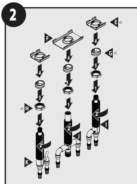
Assemble Nuts (H) Tapered Bushings (G) and Brackets (E & F) onto Valves (I & K) and Shank (J).
