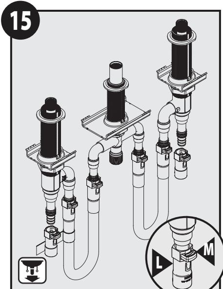
For CPVC or Cold expansion connections\*, attach the Adapters (**L** or **AA**) onto the Straight Inlet over the O-rings. Insert (**M**) into connector as shown. \* Cold expansion connectors not included.
