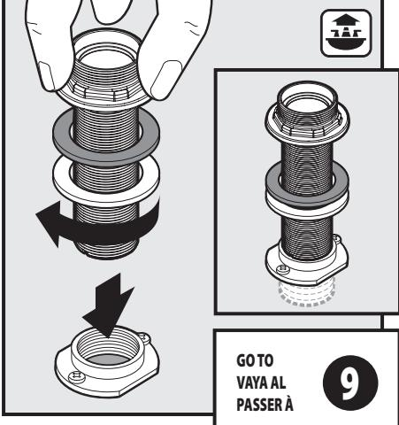
Thread Shank Assembly (Q) into Shank Adaptor (U). Leave space for planned finish deck thickness.
