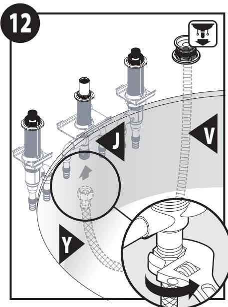
Thread Leader Hose (**Y**) onto Spout Shank (**J**) and tighten with wrench.
