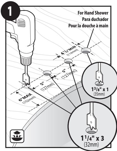
Drill 3, 1-1/4" holes for the valves and spout minimum on center. Drill a 1-3/8" hole for handshower a minimum of 4-1/2" on center to the left side of the hole for the cold valve. Position the spout hole so that spout delivers the water to the desired place in the tub.
