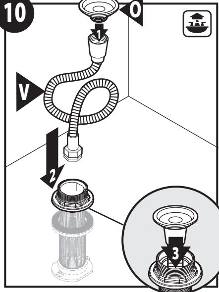
Attach Hose Retainer (O) onto Pullout Hose (V). Slide Hose into Shank.
