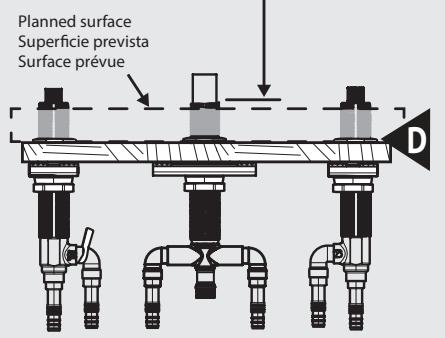
Thread Top Mounting Nuts (D) onto Spout Shank Body (J), position top threads 1/8" above planned surface height. Thread Mounting Nuts (D) onto Hot and Cold Valve Bodies (I & K). The valve body groove should be 1/8" above planned surface height.
