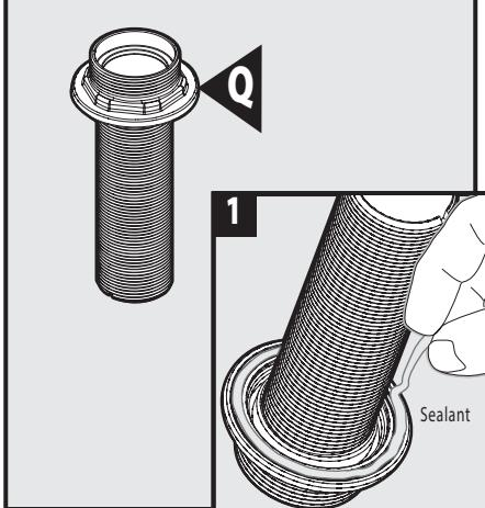
Apply sealant to underside of Plastic Adaptor (Q).
