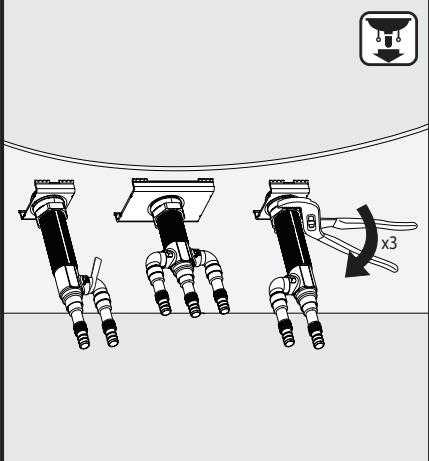
Secure Valves & Shank, tighten lower nut **firmly** using pliers.
