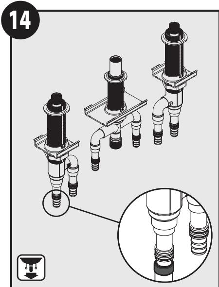
For PEX connections slide Tubing onto the Straight Inlet Tubes up to the O-ring and crimp the Banding Ring with a crimping tool.
