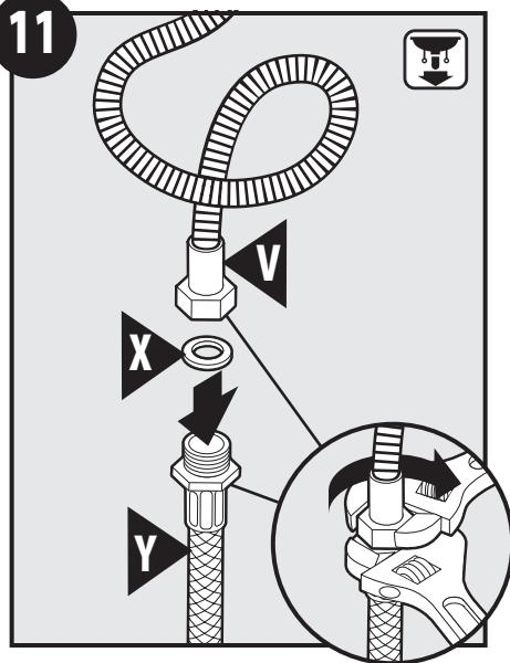
Assemble Pullout Hose (**V**) to Leader Hose (**Y**) with Washer (**X**) between fittings. Tighten with wrenches.
