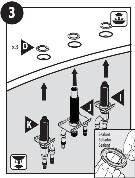
From the underside of the deck, insert completed assemblies. Position both Valve Assemblies (I & K) so the shorter legs (outlets) face towards the Center Shank Assembly (J). Add bead of sealant on bottom of top nuts.
