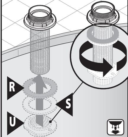
Place Gasket (R) and Washer (S) on shank under the deck and secure with Threaded Shank Adaptor.
