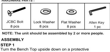
surface such as carpet or other soft material. Place the Bench Leg to corner of Apron, then tighten the Flat Washer, Lock Washer and JCBC Bolt using the Allen Key provided. Repeat the same for the other legs.
