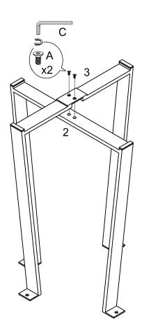
Attach part (3) to part (2) using bolt (A) with hex key (C).
