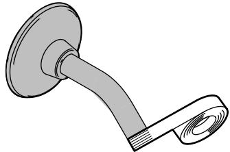
*Thread the showerhead on and tighten.*
