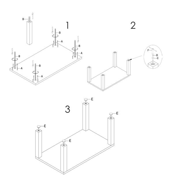
During assembly, hand tighten screws only. When all screws are in place, then tighten completely.
