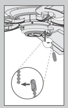
Connect the fan pull chain pendant to the short chain coming from the switch housing.
