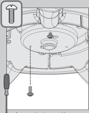
Screw two housing assembly screws from the ≡ hardware bag halfway into the motor housing. It does not matter which two screw holes you choose.
