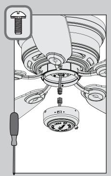
Partially install two of the switch housing screws found in the bag. Connect the plugs from the upper and lower switch housings. Make sure to line up the colored markings on the plug connectors.
