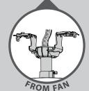
Using the orange wire connectors from the hardware bag, connect the black wire (ungrounded) from the ceiling to the black and the blue wires from the fan. Connect the white wire (grounded) from the ceiling to the white wire from the fan.
