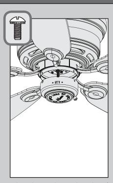
Align the notches in the sides of the lower switch housing with the screws on the upper switch housing. Twist the lower switch housing clockwise to lock into place. Install the third switch housing screw. Tighten all three screws securely.
