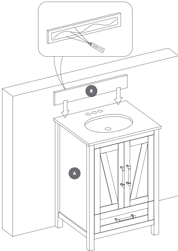
To install the top (B), apply silicone adhesive (not included) to the top edges of the vanity (A). Clean any excess adhesive before allowing to dry. Install the faucet and drain set (not included) according to the manufacturer's directions.
