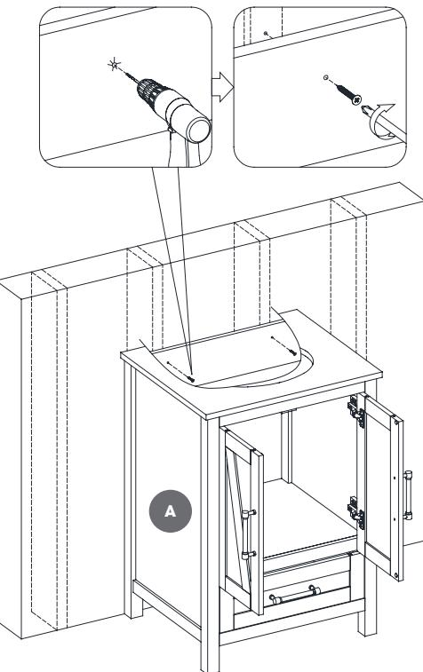
Once the desired location is chosen, temporarily move vanity (A) to the side – with the assistance of another person – and clean mounting area. Find and mark the locations of wall studs at mounting site, then replace vanity (A) in desired location. Using proper hardware (not included), drill holes at marked locations and secure vanity (A) to wall stud with at least one fastener, such as a wood screw or toggle bolt. If possible, secure vanity (A) to 2 wall studs for increased stability.
