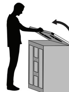
Lower the counter so that it lays flat on the cabinet, while supporting it from the side and front. Be careful not to catch your fingers under the counter. It is best to lower the counter by supporting from the front as it comes down onto the cabinet.
