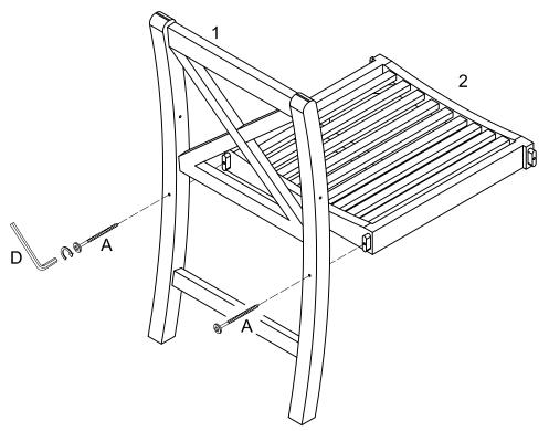
Use Wrench (D), Screw (A) to secure the Back Frame (1) to the Seat Frame (2).
