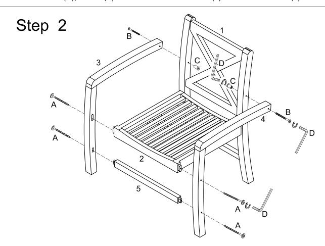
Use Wrench (D), Secure (A), Bolt (B), and Nut (C) to secure the Side Frame (3,4) to the Back Frame (1), Seat Frame (2), and Support Bar (5).
