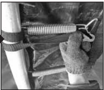
Wrap the straps on the enclosure netting (B) around the top rail (G) once around. Then, attach the strap hook to the triangle ring.
