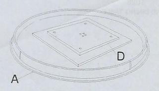
Please unscrew connecting plate D from table top and proceed with assembly as shown on the right.
