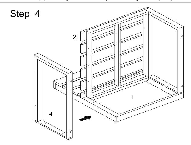
Attach right leg (4) to the back frame (1) and seat frame (2).
