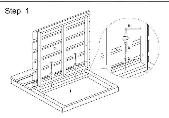
Attach seat frame (2) to the back frame (1) by using bolts (B) and washers (C). Tighten bolts (B) with wrench (E). Hands tighten the bolts only and do not tighten completely.
