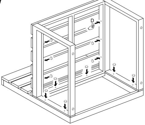
Tighten all bolts completely and cover them with the bolt caps (D).
