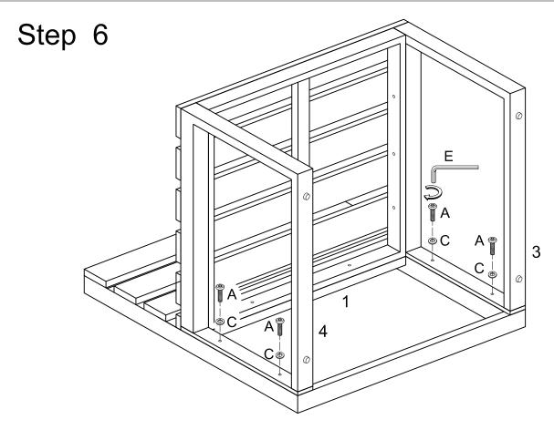
Attach left(right) leg (3, 4) to the back frame (1) by using bolts (A) and washers (C). Tighten bolts (A) with wrench (E). Hands tighten the bolts only and do not tighten completely.
