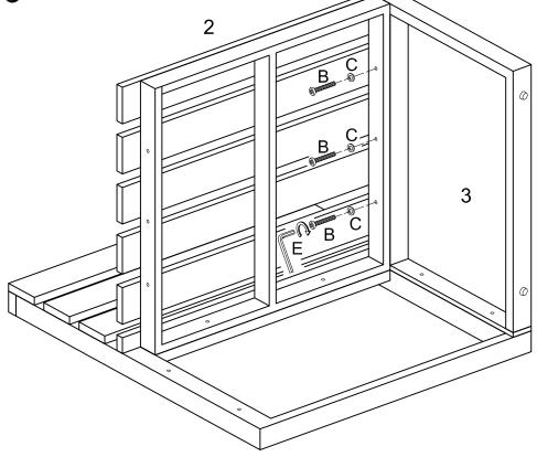
Attach left leg (3) to the seat frame (2) by using bolts (B) and washers (C). Tighten bolts (B) with wrench (E). Hands tighten the bolts only and do not tighten completely.
