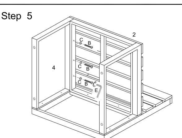
Attach right leg (4) to the seat frame (2) by using bolts (B) and washers (C). Tighten bolts (B) with wrench (E). Hands tighten the bolts only and do not tighten completely.
