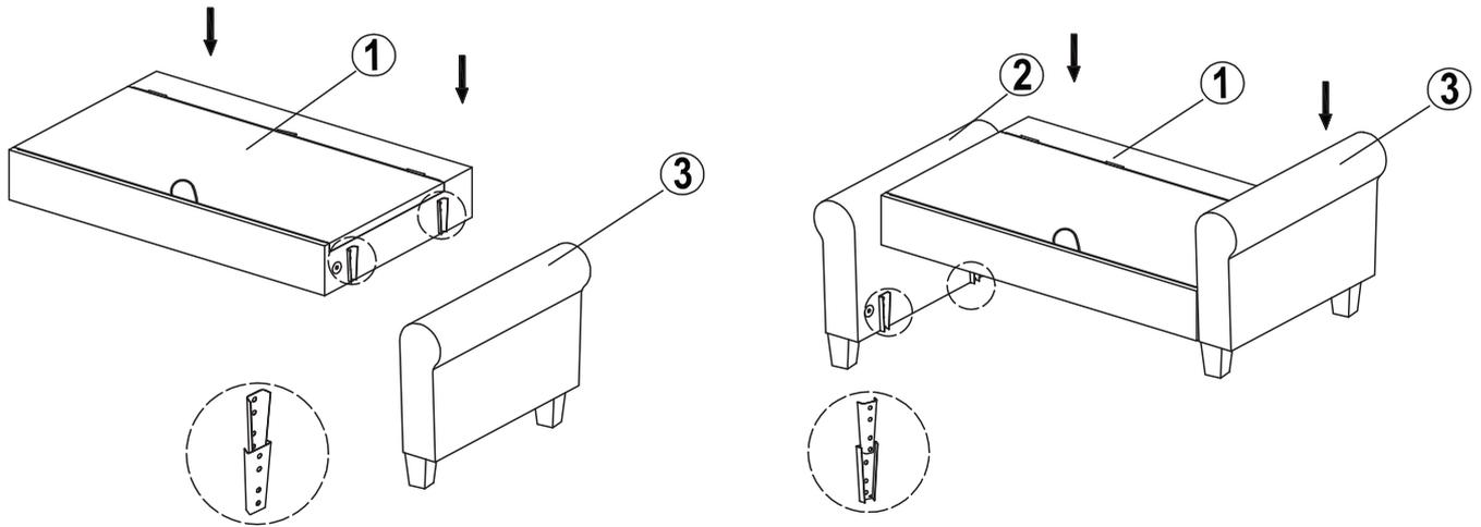
**Step 4--** 1. Open the Seat (1) bottom panel. Insert Thumb Bolts (A) x 2 into holes where sides of Seat Frame (1) and tighten the bolts to Arms (2) & (3).
