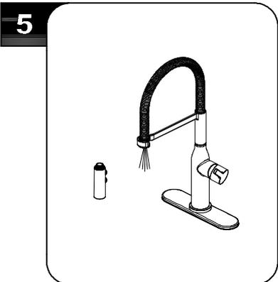
**Important:** after installation is completed, turn on hot and cold water supplies. Check for leaks. Remove the spray head by unscrewing it from the hose counterclockwise. Be sure to hold the end of the hose down into the sink and turn the faucet on to the warm position where it mixes hot and cold water. Flush water lines for one minute. Check for leaks. Re-tighten any connections if necessary, but do not overtighten. Reinstall spray head by hand tightening it back onto the spray hose.
