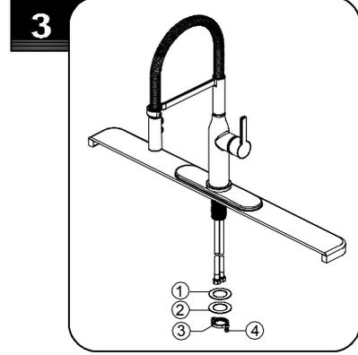
Secure the faucet assembly with the washers (1&2) and nut (3). Hand tighten the nut (3) onto the faucet assembly. Lock the nut (3) into position by tightening the screws (4) with a phillips screwdriver.
