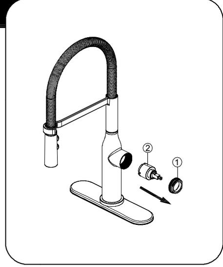
Loosen cartridge nut (1) by turning it counter-clockwise and lift out the cartridge (2). Insert new cartridge. Reinstall the handle.
