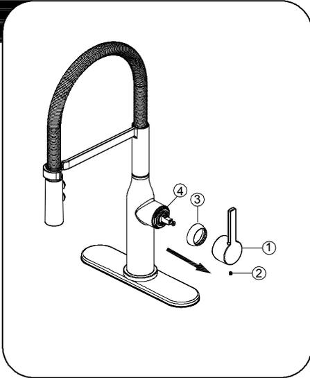
Shut off water supply. With valves in "closed" position, loosen the set screw (2) and remove handle (1). Unscrew the cap (3) from the cartridge nut (4).
