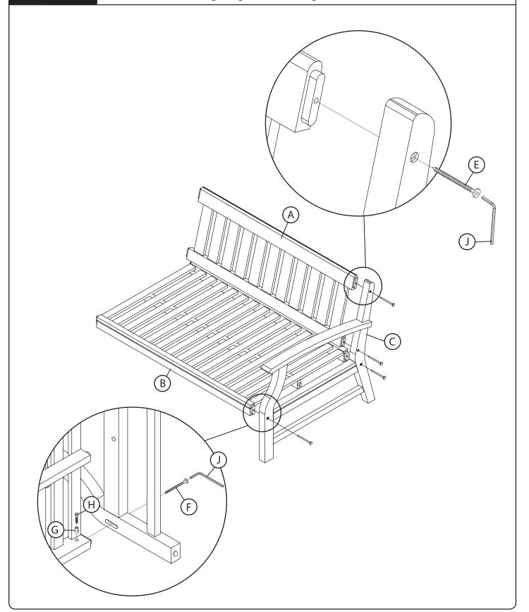
**ATTACH SEAT AND BACK TO REMAINING LEG FRAME-** Repeat steps 1 and 2 to attach seat (B) and back (A) to remaining leg frame (D).
