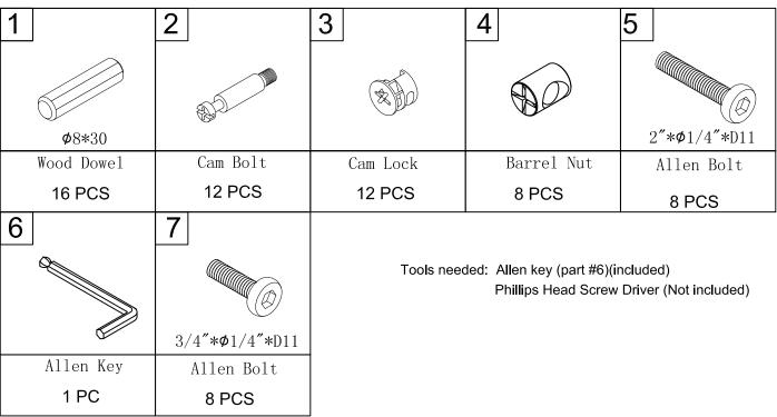
Step 1. Insert Cam Bolts (Part#2) into Top (A), Left Side Panel (B) and Right Side Panel (C).
