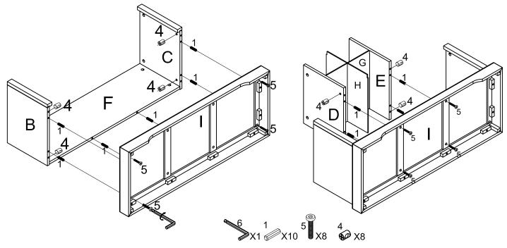
Step 4. Attach Top Panel (A) assembled (B,C,D,E,F) using Wood Dowel (Part#1) and Cam Lock (Part3).
