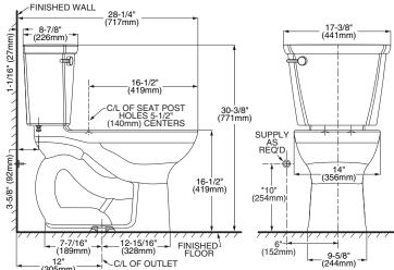
THIS TOILET IS DESIGNED TO ROUGH-IN AT A MINIMUM DIMENSION OF 305MM (12") FROM FINISHED WALL TO C/L OF OUTLET.
