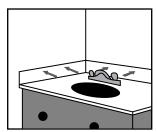
Carefully push the splash in place, making sure you firmly press it against the wall.
