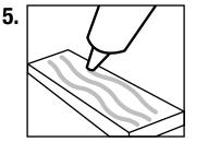
Use "Liquid Nail" or "PL Adhesive". Apply a generous amount to the back of the splash.
