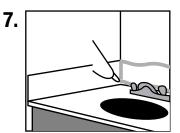
Apply "100% silicone" to the seam where the backsplash and/or sidesplash touches the granite top (indicated by grey line). Apply "kitchen & bathroom caulk" to the top edge of the splash that touches the wall.
