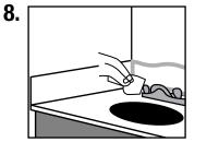
With a caulk edging tool, run it across the seams to clear away excess silicone & caulk (this technique will leave a clean line of silicone & caulk over the seams).
