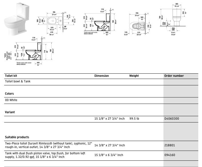
All drawings contain the necessary measurements which are subject to standard tolerances. They are stated in inch & mm and are nonbinding. Exact measurements, in particular for customized installation scenarios, can only be taken from the finished ceramic piece.
