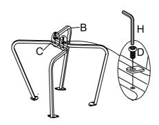
Attach base to bottom of Chair Seat (A) using Bolt (E), Spring Washer (F) and Flat Washer (G) with Allen Key (H).
