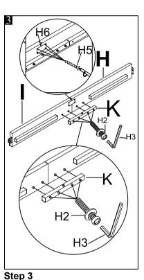
Attach wood bar "K" to the 2 rails "H" & "I".Using Allen key (H3) to lock with bolts "H2". Lock the both side rails ( H & I) (front & rear of rail) tight and alignment with metal plate (H6) by using
