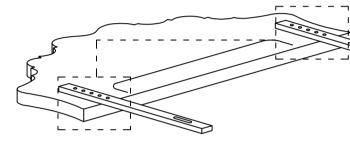
Secure each support stand by using 2x JCBB Bolt [1] and 2x M8 Flat Washer [2].
