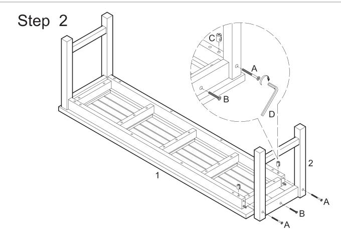
Insert barrel nuts (C) into bench seat (1). Attach leg set (2) to bench seat (1) using bolts (A,B). Bolts (A) will screw directly into barrel nuts (C). Tighten all bolts with wrench (D).
