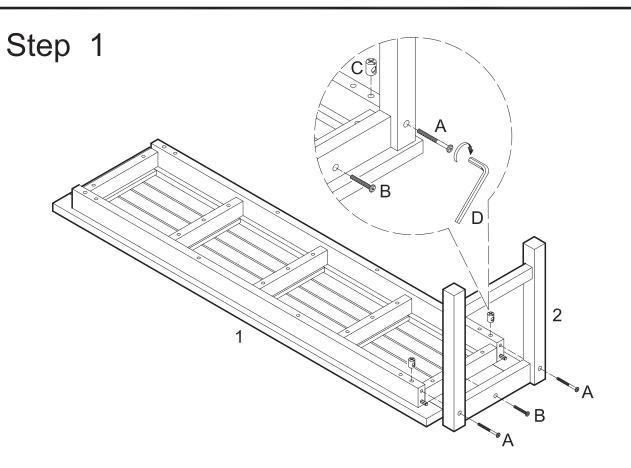
Insert barrel nuts (C) into bench seat (1). Attach leg set (2) to bench seat (1) using bolts (A,B). Bolts (A) will screw directly into barrel nuts (C). Tighten all bolts with wrench (D).
