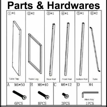
Step 1: Lay the Table Top(①) upside down onto a clean smooth surface such as carpet or cardboard. Align and fix Rear Rail(③) with 4 holes and Front Rails(④) with 2 holse to the Table Top(①) with screw(B) by Allen Key(D). Make sure the screw holes on Rear Rail(③) face up. Do not fully tighten all bolts until all parts are in place.
