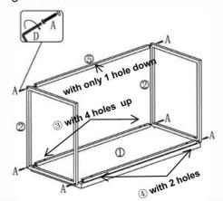
Step3: Attach and fix two support tubes(⑥) to the assembled Rear Rail(③) and Bottom Rail(⑤) by using screw(C) with supplied Allen Key(D). Tighten table legs(②) to table top by using screw (B). And then fully tighten all the screws. Flip the desk upright with the help of another person.
