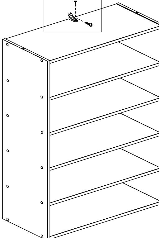
MOUNT L-BRACKET UNDERNEATH EACH TOP SHELF FOR STACKING!
