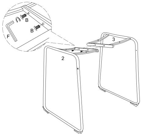
Attach the metal frame (2) to metal frame (3) by using bolts (B) and wrench (F). Do not tighten bolts completely until step #2.
