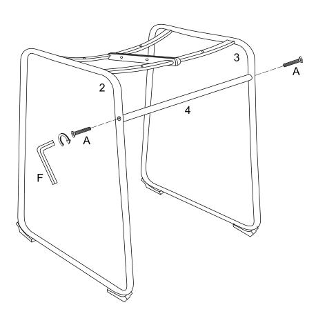
Attach the metal tubes (4) to the metal frame (2)(3) and secure it by using bolts (A) and wrench (F). Tighten bolts from assembly in Step 1.
