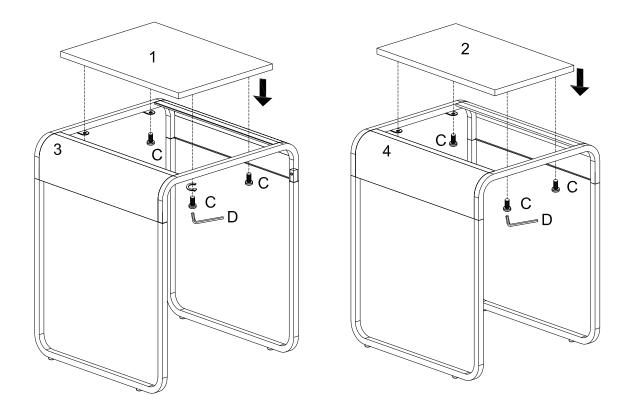
Attach part (1) to part (3), part (2) to part (4) using bolt (C) with hex key (D).
