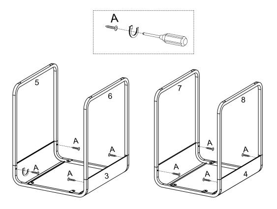
Secure part (5, 6), (7, 8) to part (3), (4) using screw (A) with head Philips screwdriver.
