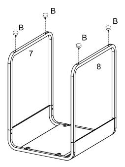
Screw adjustable foot (B) onto part (5, 6, 7, 8) per diagram.
