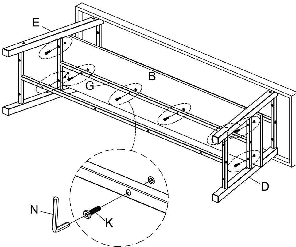
**5** Attach Bottom Panel (C) to Left Side Frame (D), Right Side Frame (E) and Bottom Cross Bar (H) using Bolt (K) by Allen Key (N) as below shown.
