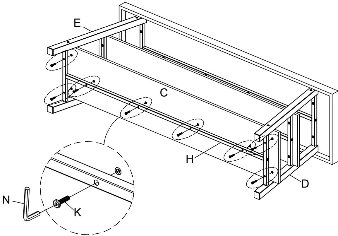
**6** Attach Back Cross Bar (I) to the back of Left Side Frame (D) and Right Side Frame (E) using Bolt (J) by Allen Key (N) to lock the bottom holes of Cross Bar (I) first only as below shown.
